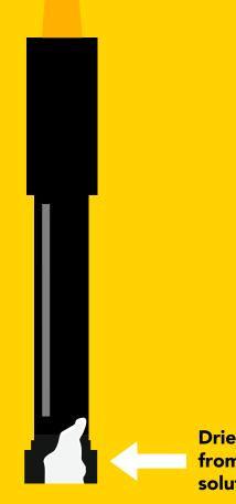
Dried KCl residue from Electrolyte solution
