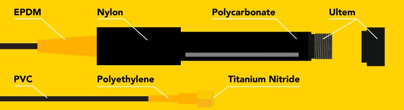
This Dissolved Oxygen probe can be fully submerged in fresh or salt water, up to the SMA connector indefinitely.
