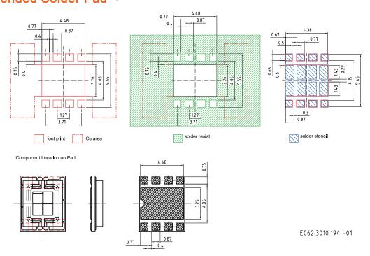
For superior solder joint connectivity results we recommend soldering under standard nitrogen atmosphere. Package not suitable for any kind of wet cleaning or ultrasonic cleaning.
