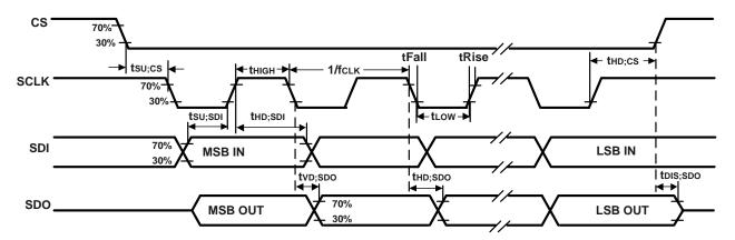
Figure 2. SPI Bus Timing Diagram
