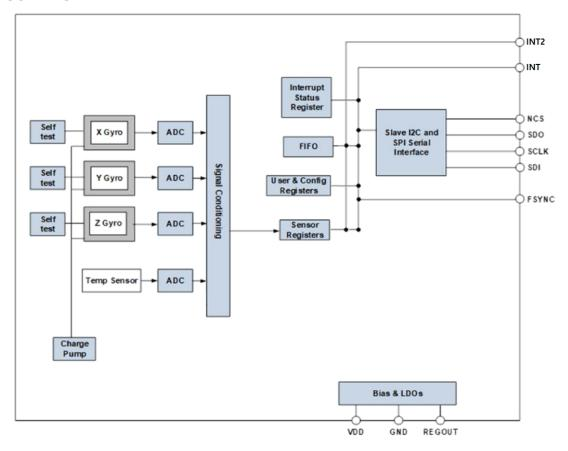
Figure 5. IAM-20380HT Block Diagram
