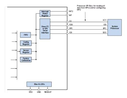
Figure 7. IAM-20380HT Solution Using SPI Interface
