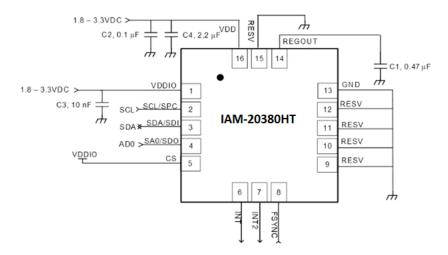
Figure 4. IAM-20380HT LGA Application Schematic
