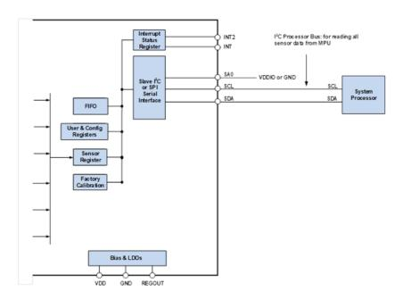
Figure 6. IAM-20380HT Solution Using I<sup>2</sup>C Interface
