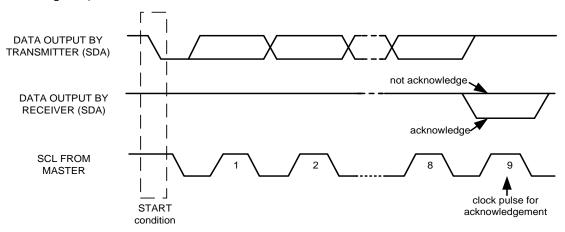
Figure 9. Acknowledge on the I<sup>2</sup>C Bus
