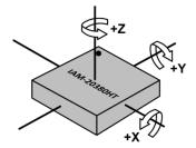
Figure 13. Orientation of Axes of Sensitivity and Polarity of Rotation
