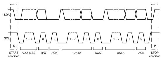
Figure 10. Complete I<sup>2</sup>C Data Transfer
