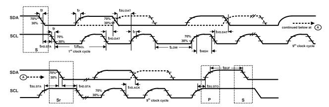
Figure 1. I<sup>2</sup>C Bus Timing Diagram
