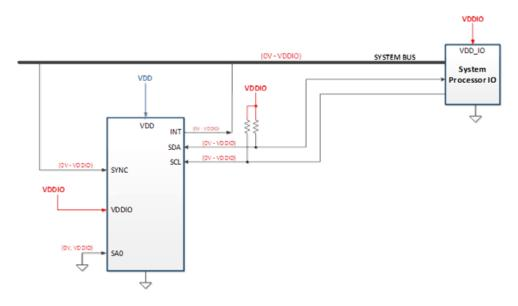
Figure 12. I/O Levels and Connections
