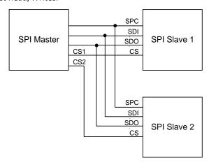
Figure 11. Typical SPI Master/Slave Configuration
