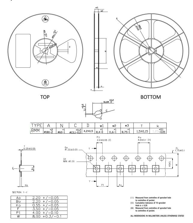
Figure 8: 8TR8211C Tape and Reel Dimension
