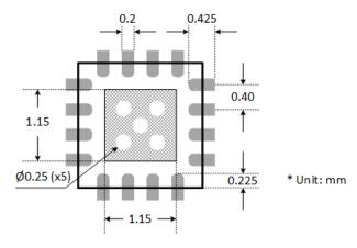
Figure 5: 8TR8211C Recommended PCB Layout Footprint
