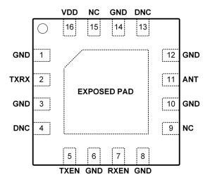
Figure 3: Pin Description (Top View)
