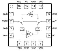
Figure 1: Functional Block Diagram
