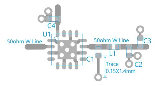
Figure 4: 8TR8211C Reference Design Schematic and PCB Layout
