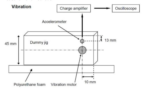
Specification of the dummy Jig
