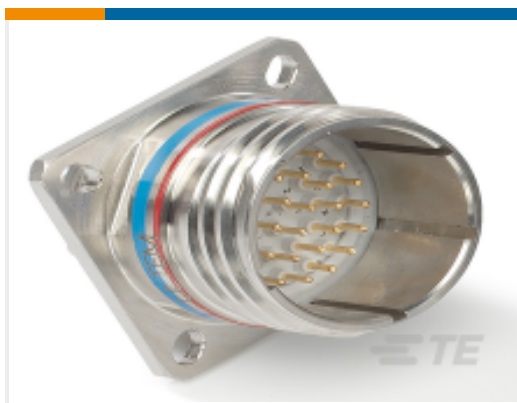
TE Part # CAT-D38999-DTS7D D38999: Square Flange, 21-11 insert
