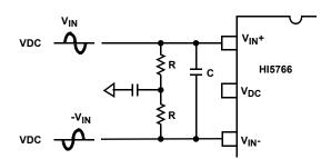
FIGURE 26. DC COUPLED DIFFERENTIAL INPUT
