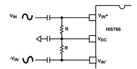
FIGURE 25. AC COUPLED DIFFERENTIAL INPUT
