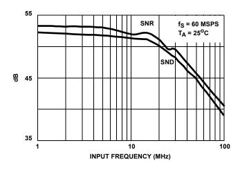
FIGURE 4. SINAD AND SNR vs INPUT FREQUENCY
