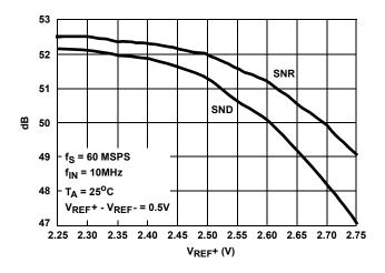
FIGURE 9. SINAD AND SNR vs  $V_{REF}$ +
