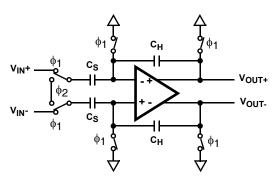
FIGURE 24. ANALOG INPUT SAMPLE-AND-HOLD
