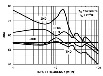
NOTE: SFDR depicted here does not include any harmonic distortion. FIGURE 5. -2HD, -3HD, -THD AND SFDR vs INPUT FREQUENCY
