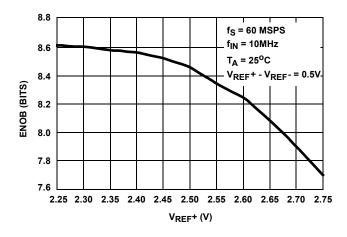
FIGURE 8. EFFECTIVE NUMBER OF BITS (ENOB) vs V<sub>REF</sub>+
