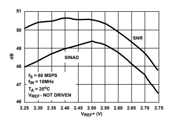
FIGURE 12. SINAD AND SNR vs V<sub>REF</sub>+ (V<sub>REF</sub>- NOT DRIVEN)
