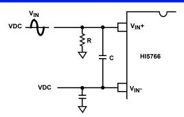
FIGURE 28. DC COUPLED SINGLE ENDED INPUT
