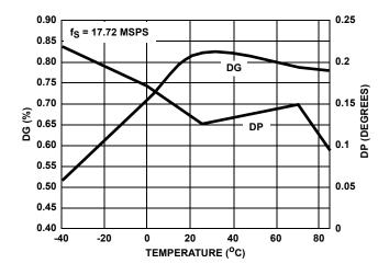
FIGURE 19. DIFFERENTIAL GAIN/PHASE vs TEMPERATURE
