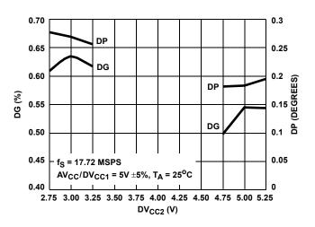
FIGURE 20. DIFFERENTIAL GAIN/PHASE vs SUPPLY VOLTAGE
