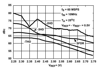
NOTE: SFDR depicted here does not include any harmonic distortion. FIGURE 10. -2HD, -3HD, -THD AND SFDR vs V<sub>REF</sub>+
