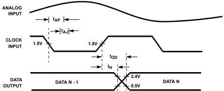
FIGURE 2. INPUT-TO-OUTPUT TIMING
