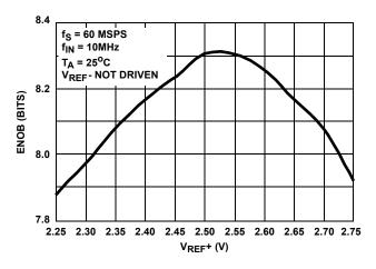
FIGURE 11. EFFECTIVE NUMBER OF BITS (ENOB) vs V<sub>REF</sub>+ (V<sub>REF</sub>- NOT DRIVEN)
