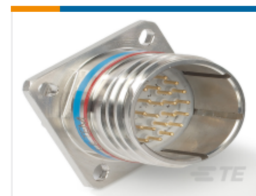
TE Part #YDTS20W11-35PAV001 D38999: Square Flange, 11-35 insert
