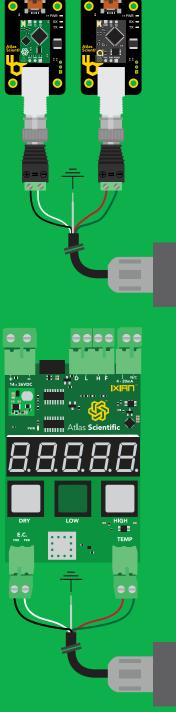
Using two **BNC with Terminal Screws**, you can easily connect the Industrial Conductivity probe to our **EZO Conductivity Circuit** and **EZO™ RTD Circuit** via our **Electrically Isolated USB EZO™ Carrier Board.**
