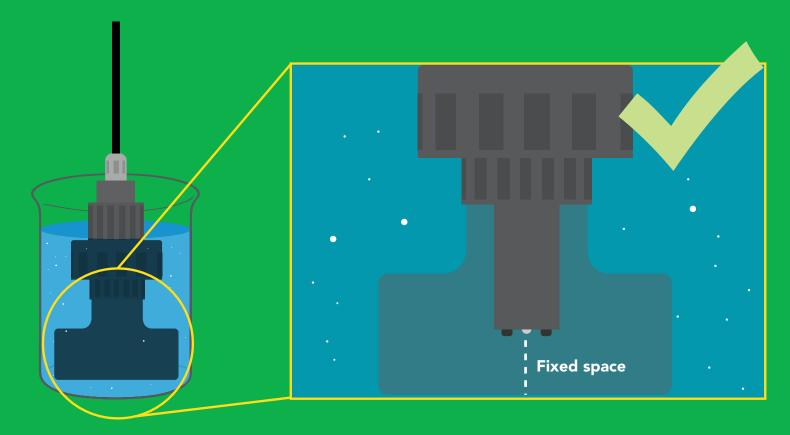
Calibrating and / or using the probe without the pipe fitting attached will cause irregular readings.
