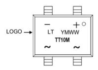
TT10M = Product Type Marking Code YMWW = Date Code Marking Y = Year Code (ex: 2 = 2022) M = Manufacturer's Internal Code WW = Week Code (01 to 53)
