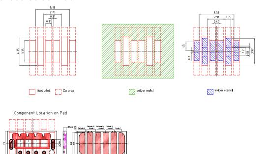
For superior solder joint connectivity results we recommend soldering under standard nitrogen atmosphere. Package not suitable for ultra sonic cleaning. To ensure a high solder joint reliability and to minimize the risk of solder joint cracks, the customer is responsible to evaluate the combination of PCB board and solder paste material for his application.
