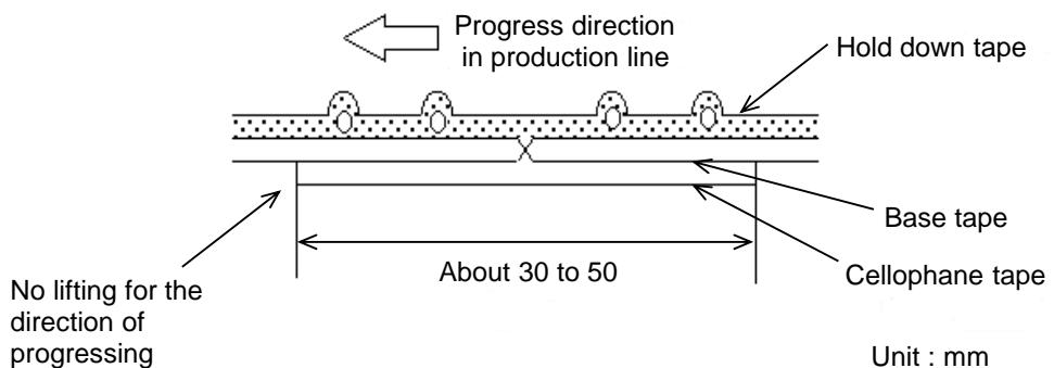
b) When hold down tape is spliced
