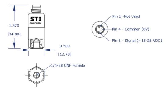
**Ordering Information:**CMCP1100C Low Cost Compact Accelerometer with M8 Connector
