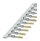
Crimp contact, Pin, rolled, Taped product, number of pieces per reel: 10000, contact diameter: 1 mm, crimp range:  $0.22 \text{ mm}^2 \dots 0.56 \text{ mm}^2$ , Item is lead-free in accordance with RoHS II without Exemption 6c (Pb < 0.1 %)
