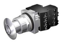
30mm Command/52, Chrome Finish Heavy Duty, Watertight/Oiltight Complete Metal Unit Illuminated Push-Pull Operator Transformer type, 600V AC Incandescent Lamp Mushroom Head Cap Small 1 3/4" (44.5 mm) Metal, Chrome with Clear Lens 3 Position Momentary 1 N.C.+1 N.C. Extra Late Break Heavy Duty Contacts, A600/P600 UL Listed, CSA Certified NEMA 1,3,3R,4,4X,12,13 & Automotive Standards
