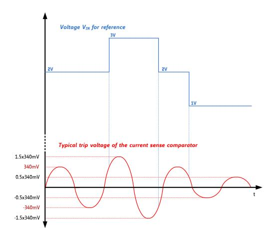
Figure 3.1 Relation between V<sub>IN</sub> and trip voltage of current sense comparator
