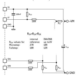
Figure 5.1 Schematic with R<sub>SH</sub>=R<sub>SA</sub>=R<sub>SB</sub>
