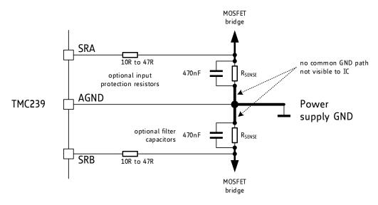
Figure 12.1 Sense resistor grounding and protection components
