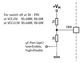
Figure 8.1 Overvoltage protection
