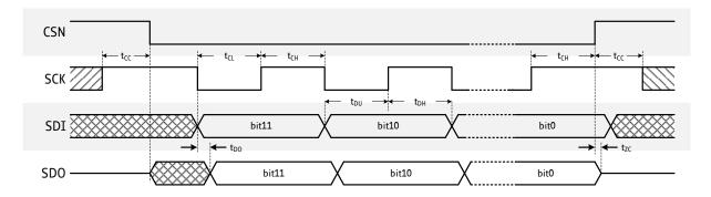
Figure 3.3 SPI Timing
