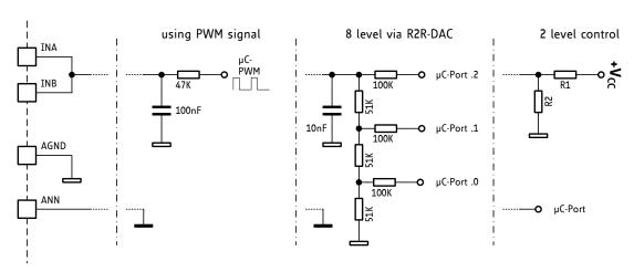
Figure 3.2 External DAC and PWM-DAC
