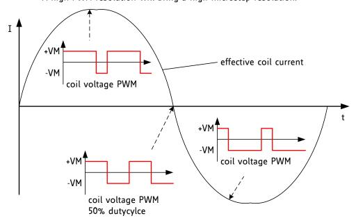
Figure 6.3 Voltage PWM generates motor current
