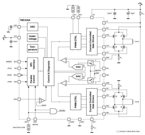
Figure 1.1 TMC239 block diagram
