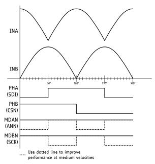
Figure 4.1 Analog control for standalone mode
