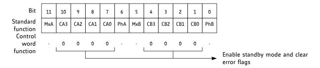
Programming current value 0000 for both coils at a time clears the overcurrent flags and switches the TMC239 into a low current standby mode with coils switched off.
