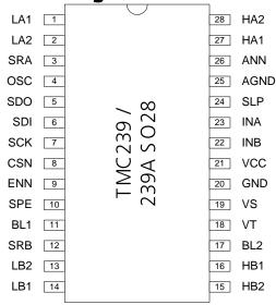
Figure 2.1 TMC239 pin assignments
