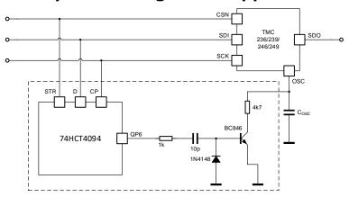
Figure 13.1 Synchronizing the chopper clock
