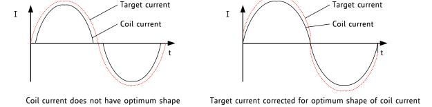
Figure 6.5 Adapting sine wave for smooth motor operation
