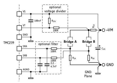
Figure 12.2 Grounding TMC239
