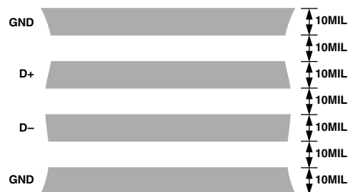
Figure 5. Arrangement of Signal Tracks
