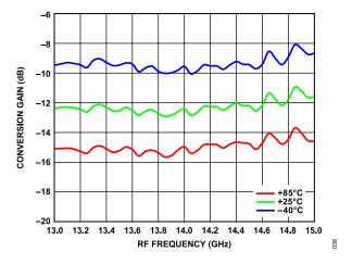
Figure 35. Conversion Gain vs. RF Frequency over Temperature
