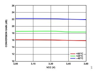
Figure 14. Conversion Gain vs. VCC over Temperature
