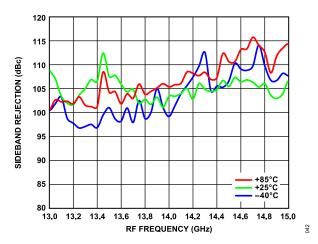
Figure 39. Sideband Rejection vs. RF Frequency over Temperature
