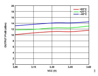
Figure 17. Output P1dB vs. VCC over Temperature
