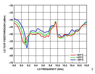
Figure 52. LO to IF Feedthrough vs. LO Frequency over Temperature
