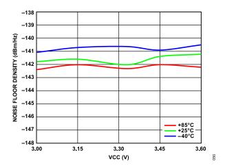
Figure 47. Noise Floor Density vs. VCC over Temperature
