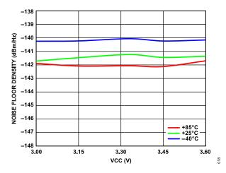
Figure 15. Noise Floor Density vs. VCC over Temperature
