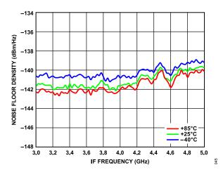
Figure 42. Noise Floor Density vs. IF Frequency over Temperature
