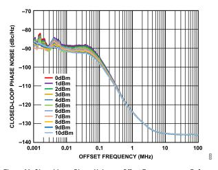
Figure 30. Closed-Loop Phase Noise vs. Offset Frequency over Reference Input Power
