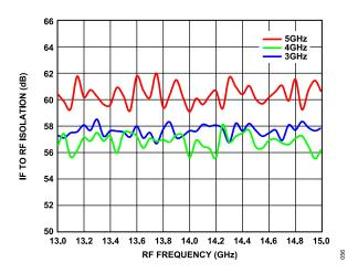
Figure 53. IF to RF Isolation vs. RF Frequency, IF = 3 GHz, 4 GHz, and 5 GHz
