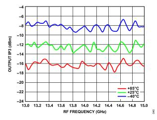
Figure 37. Output IP3 vs. RF Frequency over Temperature
