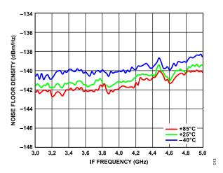
Figure 10. Noise Floor Density vs. IF Frequency over Temperature
