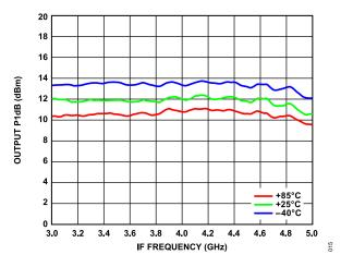
Figure 12. Output P1dB vs. IF Frequency over Temperature
