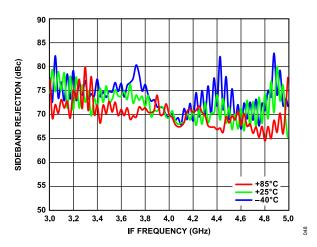
Figure 45. Sideband Rejection vs. IF Frequency over Temperature
