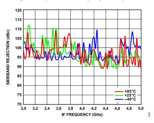
Figure 13. Sideband Rejection vs. IF Frequency over Temperature
