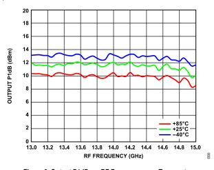
Figure 6. Output P1dB vs. RF Frequency over Temperature
