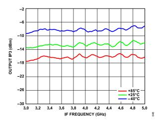
Figure 43. Output IP3 vs. IF Frequency over Temperature
