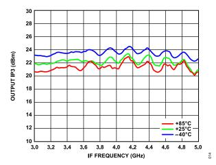
Figure 11. Output IP3 vs. IF Frequency over Temperature
