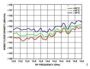
Figure 36. Noise Floor Density vs. RF Frequency over Temperature
