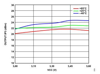
Figure 16. Output IP3 vs. VCC over Temperature
