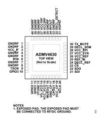
Figure 2. Pin Configuration
