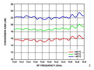
Figure 3. Conversion Gain vs. RF Frequency over Temperature
