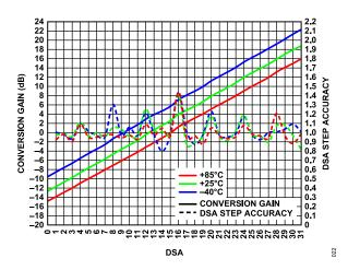
Figure 19. Conversion Gain and DSA Step Accuracy vs. DSA over Temperature
