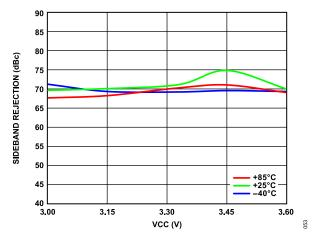
Figure 50. Sideband Rejection vs. VCC over Temperature
