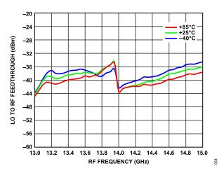
Figure 51. LO to RF Feedthrough vs. RF Frequency over Temperature
