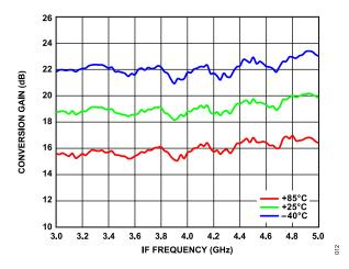
Figure 9. Conversion Gain vs. IF Frequency over Temperature
