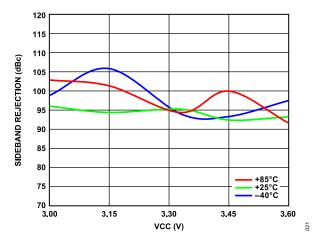
Figure 18. Sideband Rejection vs. VCC over Temperature
