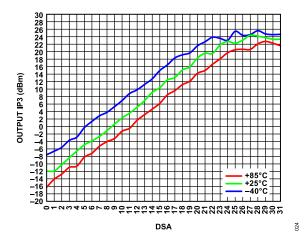
Figure 21. Output IP3 vs. DSA over Temperature
