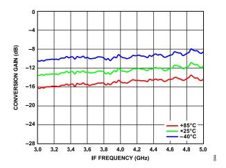
Figure 41. Conversion Gain vs. IF Frequency over Temperature
