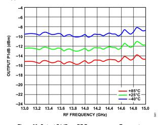
Figure 38. Output P1dB vs. RF Frequency over Temperature
