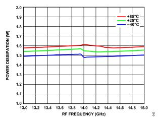
Figure 40. Power Dissipation vs. RF Frequency over Temperature
