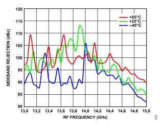
Figure 7. Sideband Rejection vs. RF Frequency over Temperature
