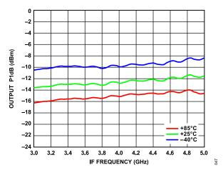
Figure 44. Output P1dB vs. IF Frequency over Temperature
