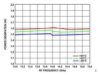
Figure 8. Power Dissipation vs. RF Frequency over Temperature
