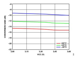
Figure 46. Conversion Gain vs. VCC Frequency over Temperature
