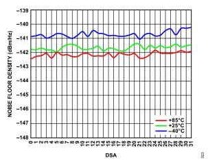
Figure 20. Noise Floor Density vs. DSA over Temperature
