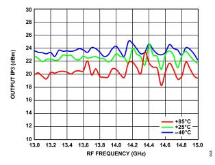
Figure 5. Output IP3 vs. RF Frequency over Temperature
