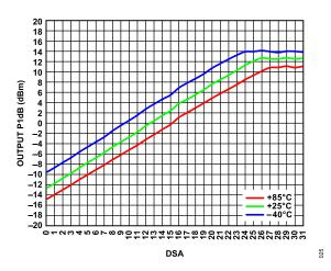
Figure 22. Output P1dB vs. DSA over Temperature
