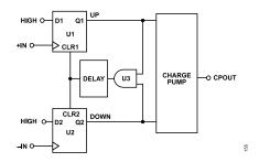
Figure 56. PFD and CP Simplified Schematic
