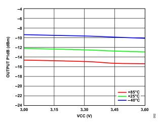
Figure 49. Output P1dB vs. VCC over Temperature
