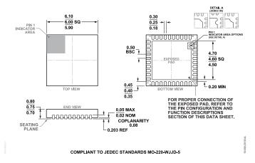
Figure 59. 40-Lead Lead Frame Chip Scale Package [LFCSP]
