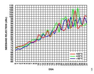
Figure 23. Sideband Rejection vs. DSA over Temperature
