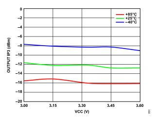
Figure 48. Output IP3 vs. VCC over Temperature
