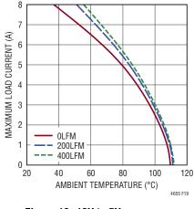
Figure 19. 12V to 5V<sub>OUT</sub> Derating Curve, No Heat Sink <sub>Rev. B</sub>
