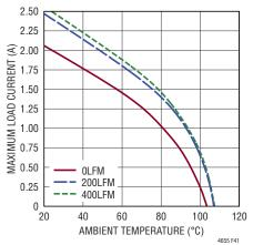
Figure 41. 12V to -24V<sub>OUT</sub> Derating Curve, No Heat Sink
