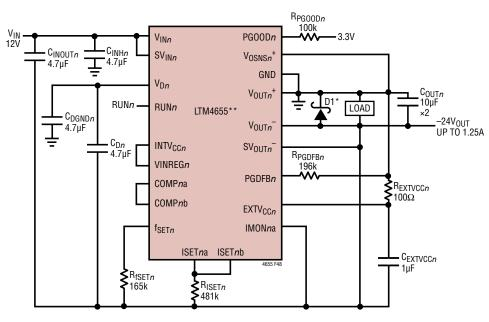
\*D1 OPTIONAL (SEE EFFECT IN FIGURE 49): CENTRAL SEMICONDUCTOR P/N CMMSH1-40L \*\*ONE CHANNEL SHOWN. PINS NOT USED AND NOT SHOWN IN THIS CIRCUIT: NC, SV<sub>INFn</sub>, IMON*n*b, LDO<sub>IN</sub>, LDO<sub>OUT</sub>, CLKSET, MOD, CLKOUT*n*, CLKIN*n*, TEMP<sup>+</sup>, TEMP<sup>-</sup>
