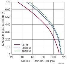
Figure 30. 24V to –5V<sub>OUT</sub> Derating Curve, No Heat Sink
