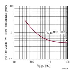
Figure 1. Relationship Between  $R_{fSETn}$  and Target  $f_{SWn}$
