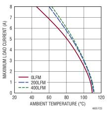
Figure 22. 24V to 5V<sub>OUT</sub> Derating Curve, with BGA Heat Sink
