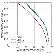
Figure 33. 24V to –5V<sub>OUT</sub> Derating Curve, with BGA Heat Sink
