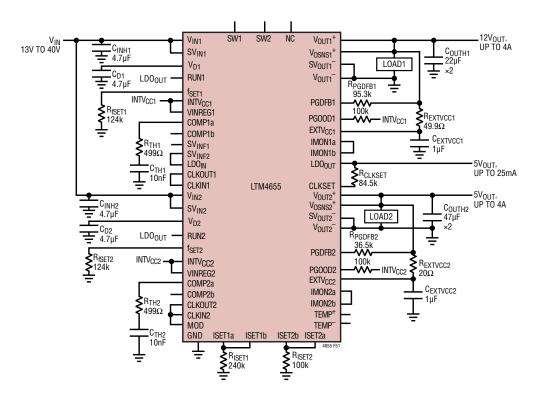
Figure 51. Dual 4A, 12V and 5V Output DC/DC µModule Regulator
