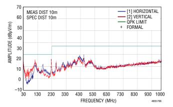
Figure 7. Radiated Emissions Scan of the LTM4655. Producing  $24V_{OUT}$  at 7A, from  $36V_{IN}$ . DC2898A Hardware.  $f_{SW}$  = 1.2MHz. Measured in a 10m Chamber. Peak Detect Method
