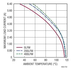
Figure 32. 12V to  $-5V_{OUT}$  Derating Curve, with BGA Heat Sink
