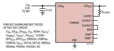
Test Circuit 3. Clock-Generator, 5V LDO and Temperature-Sensor
