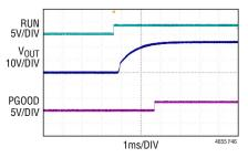
Figure 46. Start-Up Waveforms at  $36V_{IN}$ , Figure 45 Circuit
