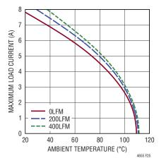
Figure 23. 24V to  $15V_{\mbox{OUT}}$  Derating Curve, No Heat Sink
