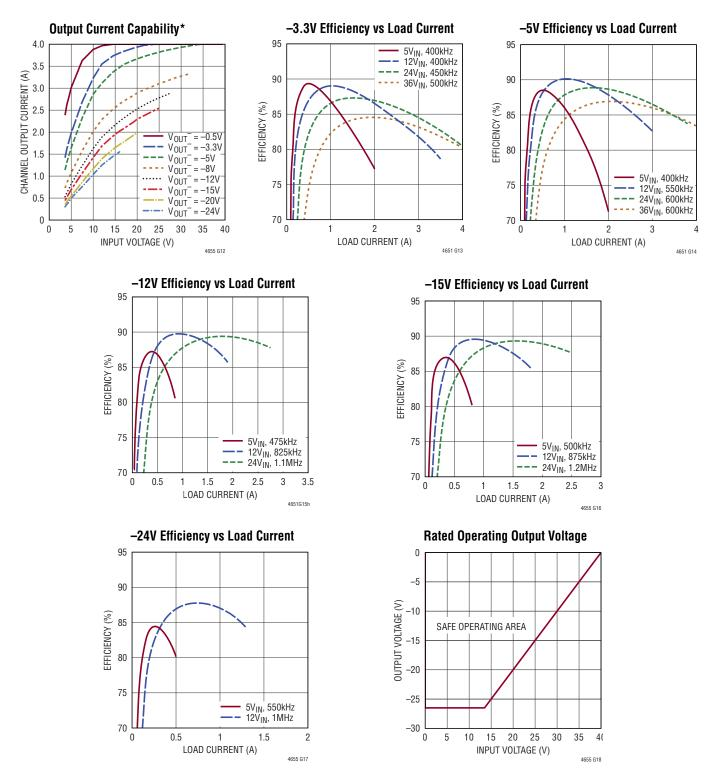
\*Current limit frequency-foldback activates at load currents higher than indicated curves. Continuous channel output current capability subject to details of application implementation. Switching frequency set per Table 1. See Notes 2 and 3.
