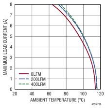
Figure 16. 5V to  $1V_{\text{OUT}}$  Derating Curve, with BGA Heat Sink
