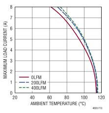
Figure 13. 5V to  $1V_{OUT}$  Derating Curve, No Heat Sink
