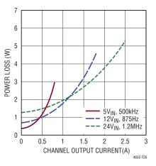
Figure 26. –15V<sub>OUT</sub> Power Loss Curve
