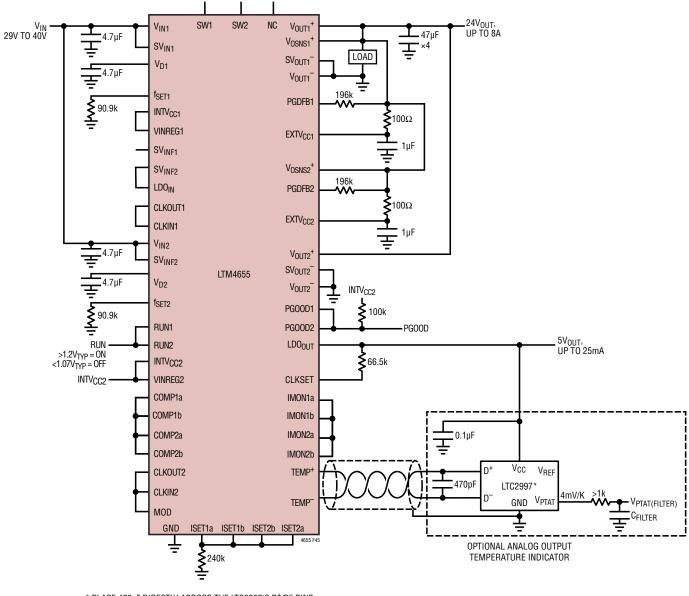
\* PLACE 470pF DIRECTLY ACROSS THE LTC2997'S D<sup>+</sup>/D<sup>-</sup> PINS. ROUTE TEMP<sup>+</sup>/TEMP<sup>-</sup> DIFFERENTIALLY TO D<sup>+</sup>/D<sup>-</sup> AND PROTECT FROM NOISE WITH GROUND SHIELDING. TERMINATE (CONNECT) THE D<sup>+</sup>/D<sup>-</sup> GROUND SHIELD AT THE LTC2997 GND PIN, ONLY. FOR BEST V<sub>PTAT</sub> PERFORMANCE, THE V<sub>CC</sub> PIN OF THE LTC2997 MUST BE LOCALLY BYPASSED AND QUIET. SEE LTC2997 DATA SHEET AND APRIL 2017 LT JOURNAL TECHNICAL ARTICLES.
