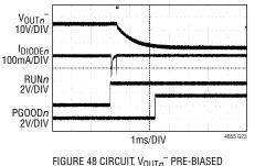
FIGURE 48 CIRCUIT, V<sub>OUT</sub>, PRE-BIASED TO –5V THROUGH A 1N4148 DIODE PRIOR TO RUN*n* TOGGLING HIGH
