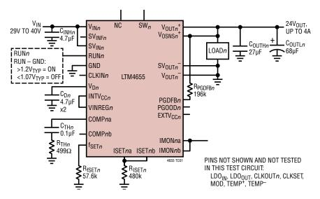
Test Circuit 1. Positive-V<sub>OUT</sub> Configuration, Regulating V<sub>OUT $n^+$ </sub>, One Channel Shown
