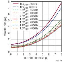
Figure 12. 24V<sub>IN</sub> Power Loss Curve
