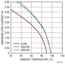
Figure 39. 24V to  $-15V_{OUT}$  Derating Curve, with BGA Heat Sink
