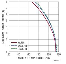
Figure 14. 12V to 1V<sub>OUT</sub> Derating Curve, No Heat Sink
