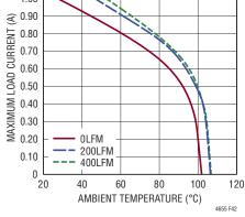
Figure 42. 5V to -24V<sub>OUT</sub> Derating Curve, with BGA Heat Sink
