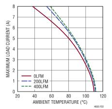
Figure 21. 12V to 5V<sub>OUT</sub> Derating Curve, with BGA Heat Sink
