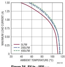
Figure 34. 5V to –15V<sub>OUT</sub> Derating Curve, No Heat Sink
