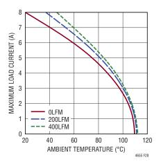
Figure 24. 24V to  $15V_{OUT}$  Derating Curve, with BGA Heat Sink
