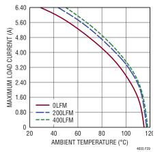
Figure 29. 12V to –5V<sub>OUT</sub> Derating Curve, No Heat Sink
