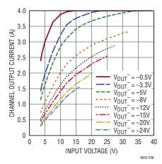
Figure 6. Channel Output Current Capability\*, Negative-V<sub>OUT</sub> Operation
