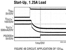
FIGURE 48 CIRCUIT, APPLICATION OF  $12V_{IN}$ , START-UP INTO 19.2 $\Omega$  LOAD
