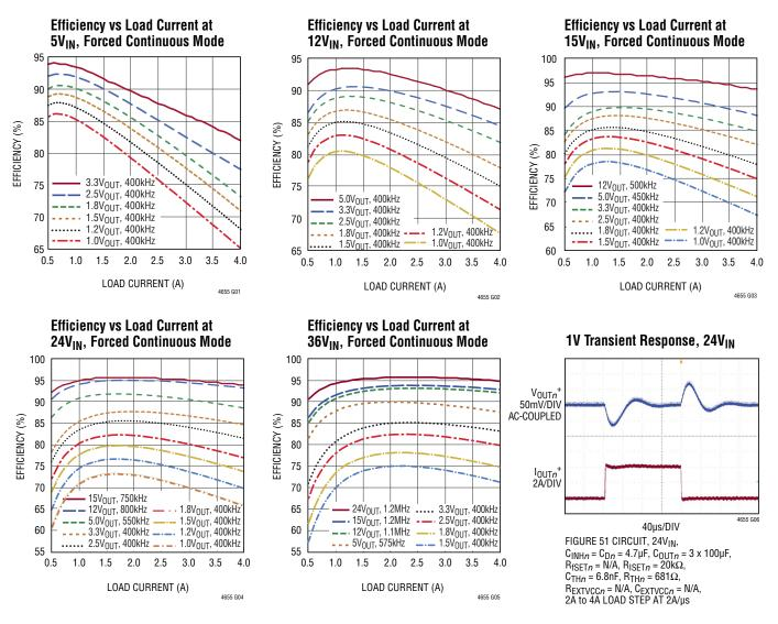
$T_A = 25^{\circ}C$ , single channel positive- $V_{OUTn}^+$  operation only, unless otherwise noted.
