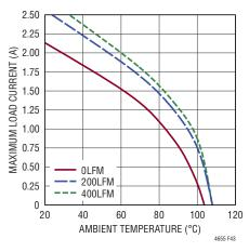
Figure 43. 12V to -24V<sub>OUT</sub> Derating Curve, with BGA Heat Sink
