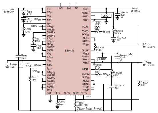
Figure 50. Concurrent ±12V Output DC/DC µModule Regulator
