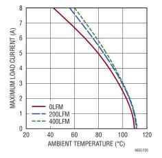
Figure 20. 24V to 5V<sub>OUT</sub> Derating Curve, No Heat Sink
