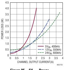
Figure 25. –5V<sub>OUT</sub> Power Loss Curve
