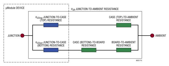
Figure 10. Graphical Representation of JESD51-12 Thermal Coefficients
