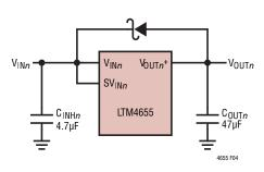
Figure 4. Schottky Diode from  $V_{OUTn}^+$  to  $V_{INn}$
