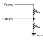
Figure 2. Undervoltage Lockout Resistive Divider
