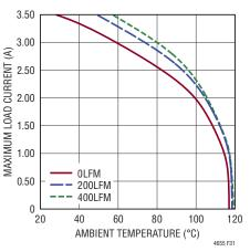
Figure 31. 5V to –5V<sub>OUT</sub> Derating Curve, with BGA Heat Sink
