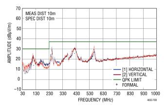
Figure 8. Radiated Emissions Scan of the LTM4655. Producing  $-24V_{OUT}$  at 2A, from  $12V_{IN}$ , DC2899A Hardware.  $f_{SW}$  = 1.2MHz. Measured in a 10m Chamber. Peak Detect Method
