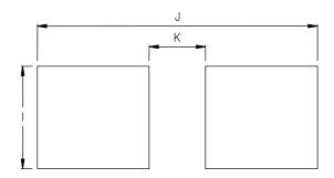
**Recommended Soldering Pad Layout**
