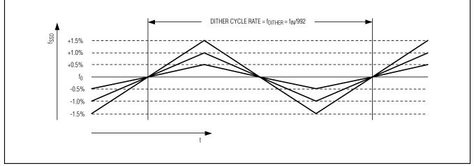
Figure 1. Spread-Spectrum Frequency Modulation
