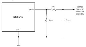
PIC 2: Charge current monitor circuit
