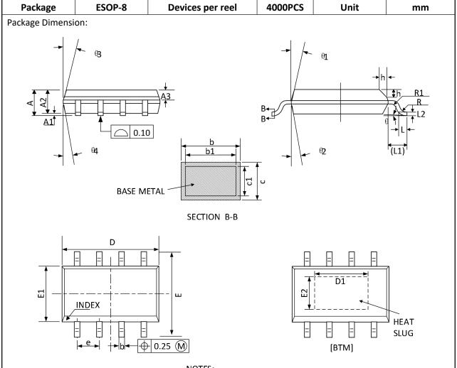
NOTES: ALL DMENSIONS REFER TO JEDEC STANDARD MS-012 AA DO NOT INCLUDE MOLD FLASH OR PROTRUSIONS.
