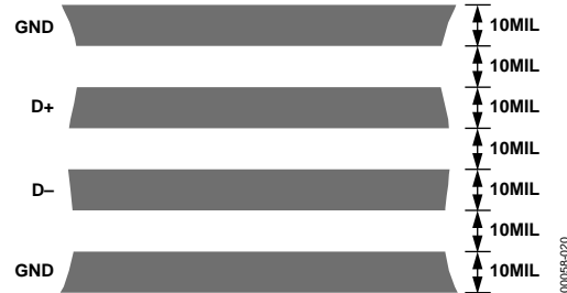
Figure 20. Arrangement of Signal Tracks
