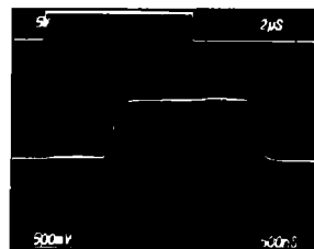
MUX-08 SMALL-SIGNAL SWITCHING WITH FILTERING AND 2.5μs SAMPLE TIME
