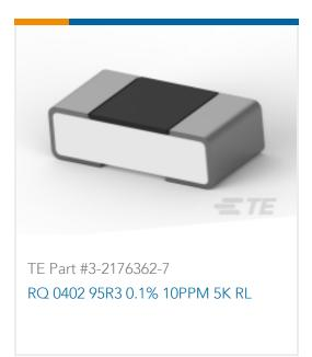
261  $\Omega$ , Thin Film, Precision Resistor, .1 %, 2 Termination, 0402, Taped & Reeled, .0625 W,  $\pm 10$  ppm/°C, Solder, Height .012 in [.3 mm], Holsworthy RQ73
