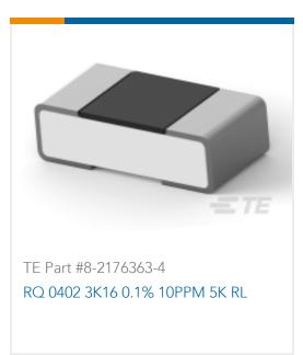
3.16K  $\Omega$ , Thin Film, Precision Resistor, .1 %, 2 Termination, 0402, Taped & Reeled, . 063 W,  $\pm 10$  ppm/°C, Solder, Height .012 in [.3 mm], Holsworthy RN73
