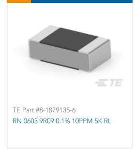
7.15  $\Omega$ , Thin Film, Precision Resistor, .1 %, 2 Termination, 0603, Taped & Reeled, .063 W,  $\pm 10$  ppm/°C, Solder, Height .018 in [.45 mm], Holsworthy RN73
