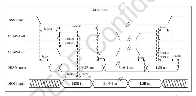
Figure 1-9. SPI Sequence Diagram - Slave Model and CPHA=1<sup>(1)</sup>
