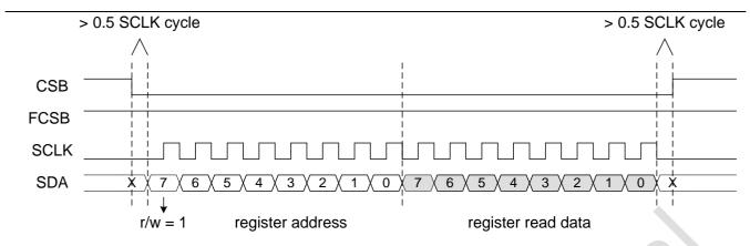
Figure 4-5. SPI Read Register Timing
