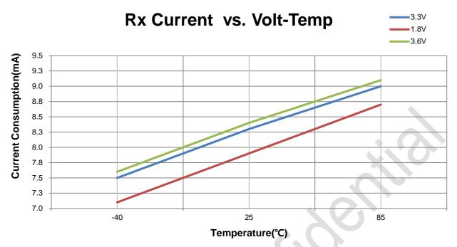
Test Condition: Freq = 434 MHz, Fdev = 10 KHz, BR = 10 Kbps
