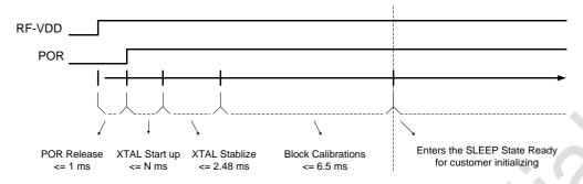
Figure 4-11. Power On Timing
