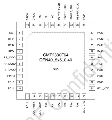
Figure 2-1. CMT2380F64-EQR Pin Diagram
