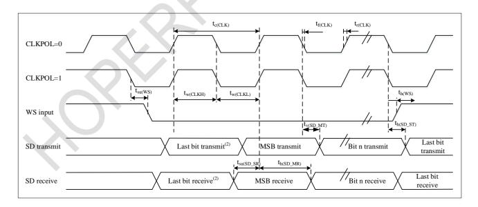
Figure 1-12. I<sup>2</sup>S Master Mode Timing Diagram (Philips protocol)<sup>(1)</sup>
