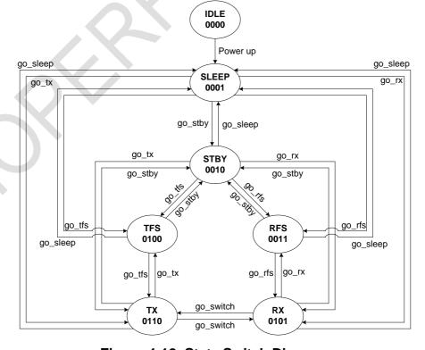
Figure 4-12. State Switch Diagram
