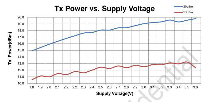
Test Condition: Freq = 434 MHz, 20 dBm / 13 dBm matching network
