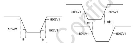
Figure 1-5. I/O AC Characteristic Definition
