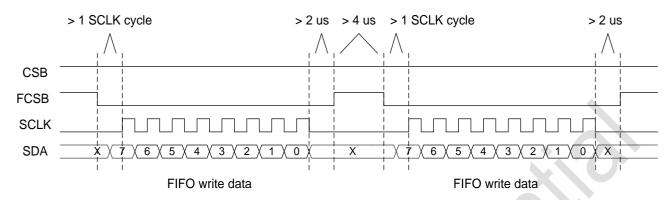
Figure 4-8. SPI Write FIFO Timing
