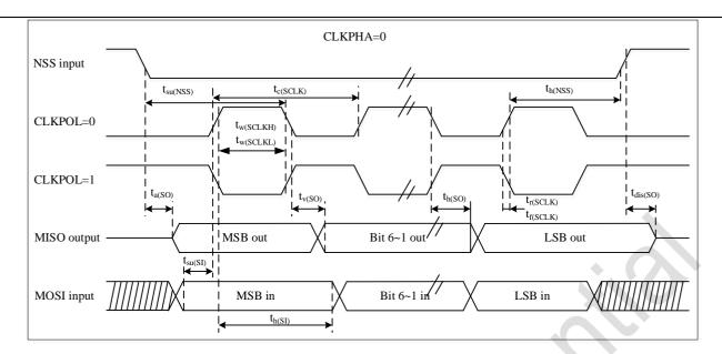
Figure 1-8. SPI Sequence Diagram - Slave Mode and CPHA=0
