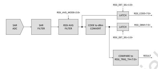
Figure 4-3. RSSI Detection and Comparison Circuit
