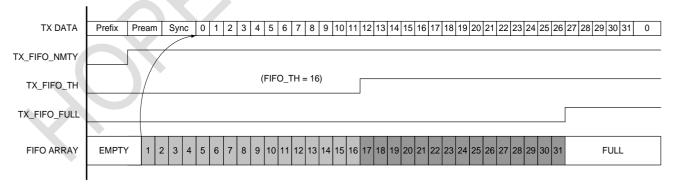
Figure 4-9. Transceiver TX FIFO Interrupt Sequence Diagram
