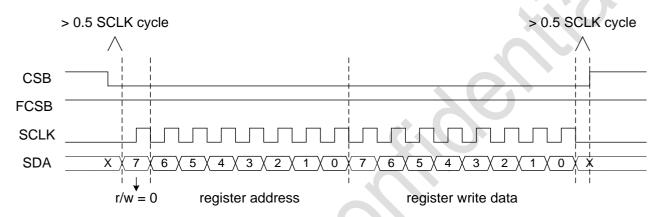
Figure 4-6. SPI Write Register Timing
