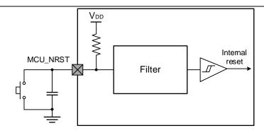
Figure 1-6. NRST Pin Protection Recommended Circuit Design
