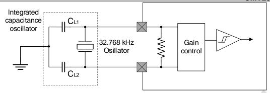
Figure 1-4. Typical Applications of Using 32.768 Khz Crystals
