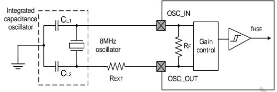
Figure 1-3. Typical Applications of Using 8MHz Crystals
