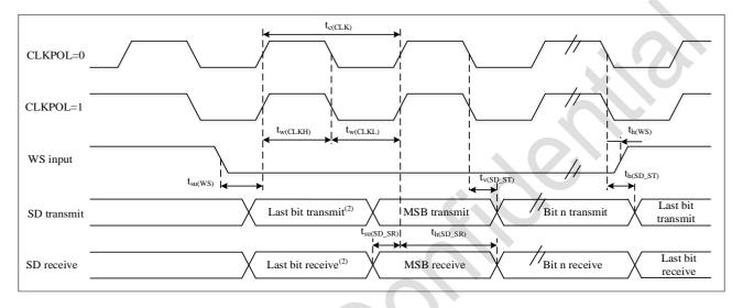
Figure 1-11. I<sup>2</sup>S Slave Mode Timing Diagram (Philips protocol)<sup>(1)</sup>
