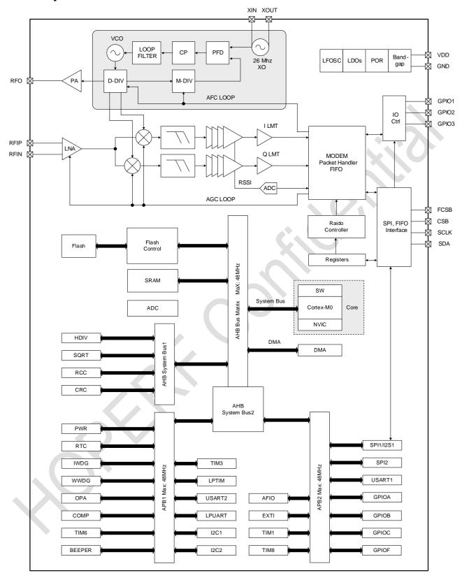
Figure 3-1. Functional Block Diagram
