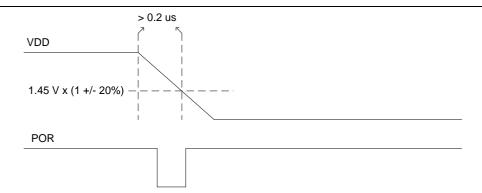
Figure 4-2. POR Reset Causing from Slow Decreasing
