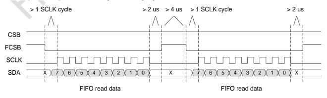
Figure 4-7. SPI Read FIFO Timing
