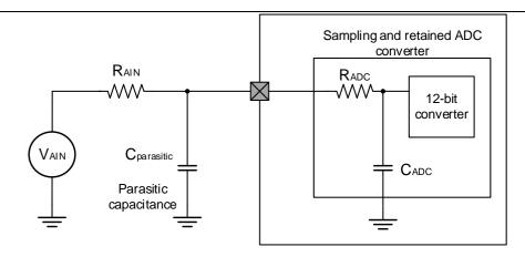
**Figure 1-13. ADC Typical Connection Diagram**
