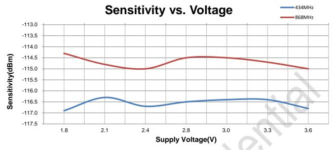
Test Condition: FSK modulation, DEV = 10 KHz, BR = 10 Kbps
