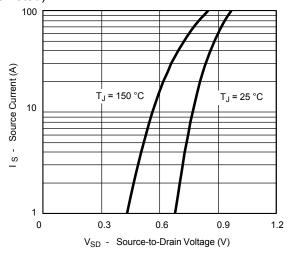
Source-Drain Diode Forward Voltage
