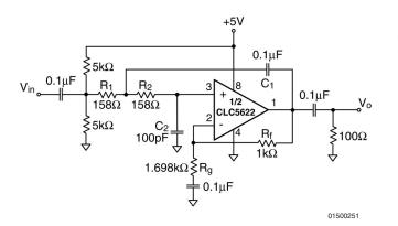
FIGURE 12. Lowpass Filter Topology
