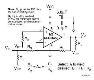
**FIGURE 2. Inverting Configuration**
