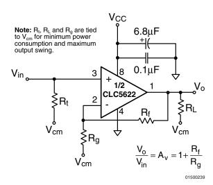
**FIGURE 1. Non-Inverting Configuration**
