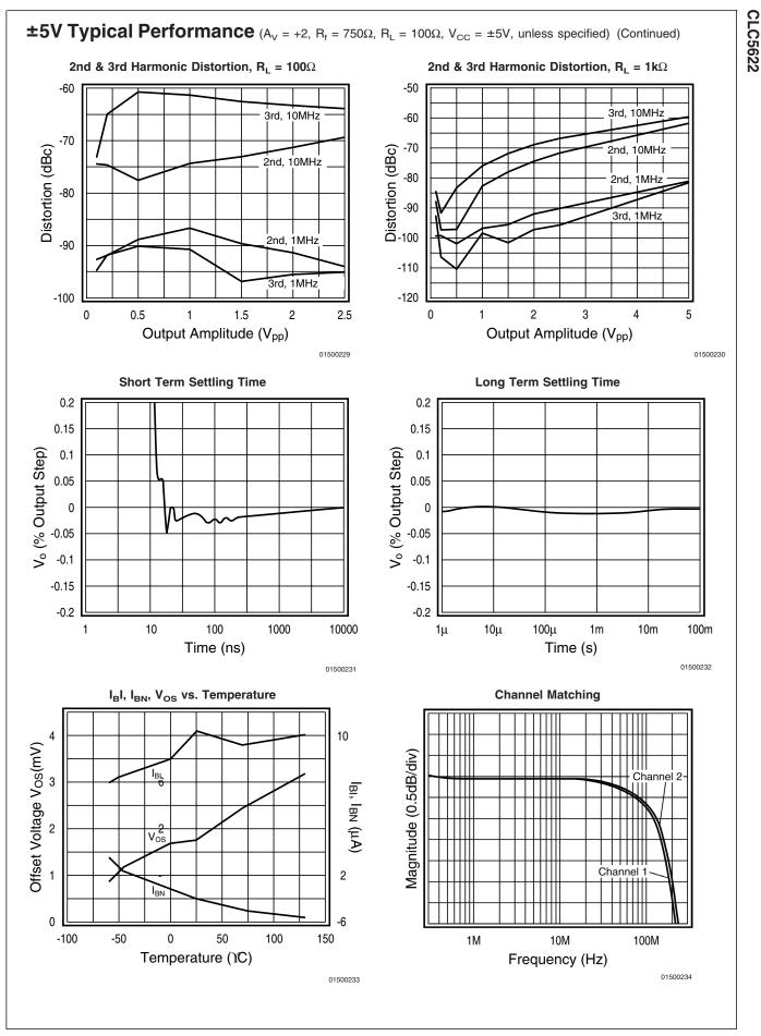
$\pm$ 5V Typical Performance (A<sub>V</sub> = +2, R<sub>f</sub> = 750 $\Omega$ , R<sub>L</sub> = 100 $\Omega$ , V<sub>CC</sub> =  $\pm$ 5V, unless specified) (Continued)
