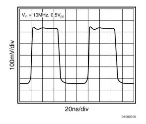
FIGURE 11. Response After 10m of Cable
