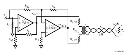
Differential Line Driver with Load Impedance Conversion
