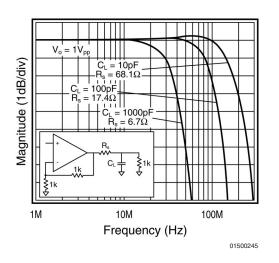
FIGURE 7. Frequency Response vs. CL
