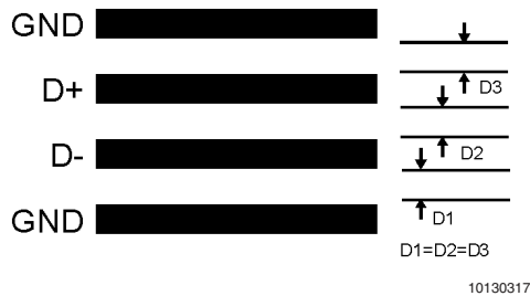
FIGURE 15. Ideal Diode Trace Layout
