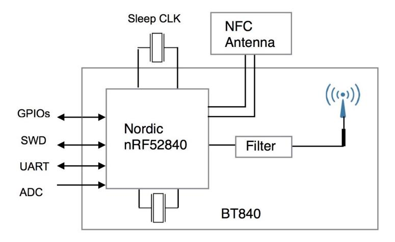
BlurNor BT840F is a sister module of BT832F. The physical size is the same. There are 21 additional LGA pins for additional GPIOs provided by nRF52840.
