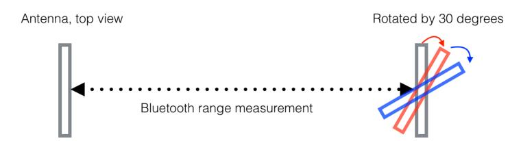
Bluetooth range is specified as the average of 12 measurements with the least significant digit truncated.
