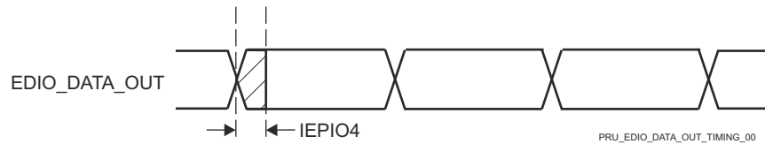
Figure 7-111. PRUSS IEP Digital IOs Timing Requirements
