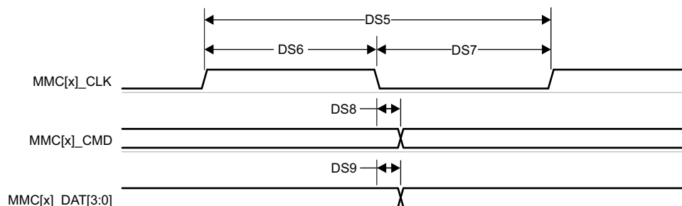
Figure 7-73. MMC0 – Default Speed – Transmit Mode
