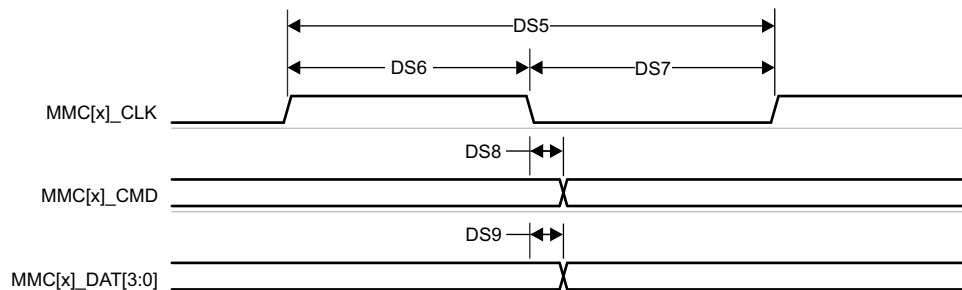
Figure 7-84. MMC1/MMC2 – Default Speed – Transmit Mode
