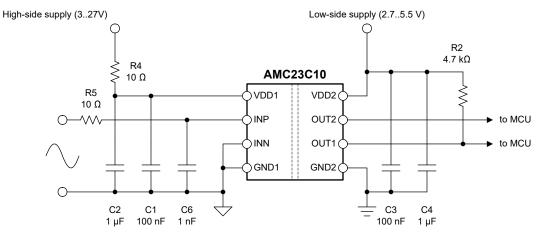
Figure 8-6. Decoupling of the AMC23C10
