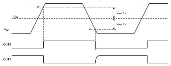
Figure 7-1. Switching Thresholds and Hysteresis
