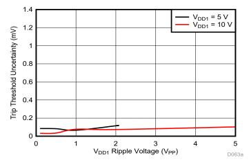
Figure 8-5. Trip Threshold Sensitivity to VDD1 Ripple Voltage (f<sub>RIPPLE</sub> = 10 kHz)
