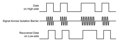
Figure 7-2. OOK-Based Modulation Scheme
