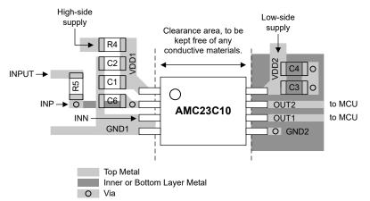
Figure 8-7. Recommended Layout of the AMC23C10
