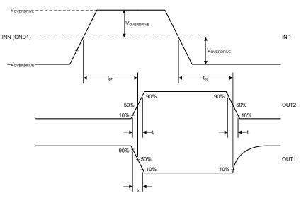
Figure 6-1. Rise, Fall, and Delay Time Definition
