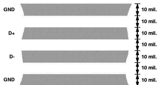
Figure 17. Arrangement of Signal Tracks
