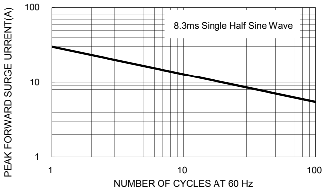
FIG. 3 MAXIMUM NON-REPETITIVE FORWARD SURGE CURRENT
