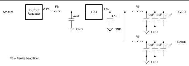
Figure 9-8. Example: LDO Linear Regulator Approach
