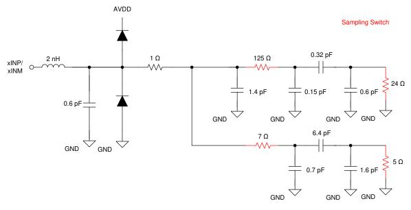
Figure 8-1. Equivalent Input Network
