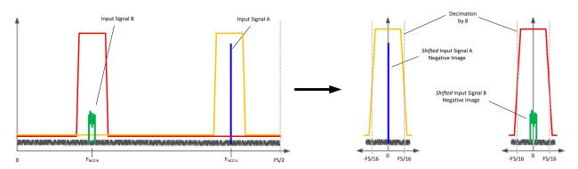
Figure 8-23. Complex Decimation (by 8) with dual band illustration
