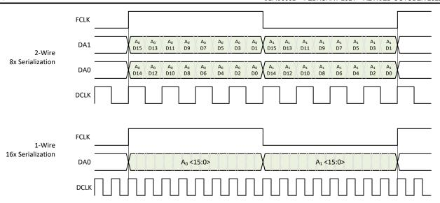
Figure 8-40. Output Data Format in Real Decimation
