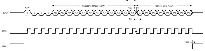
Figure 8-53. Serial Register Read Timing Diagram
