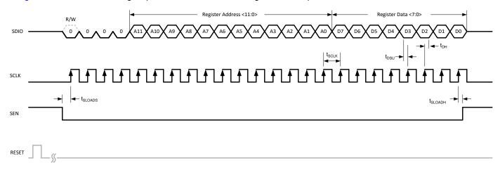
Figure 8-52. Serial Register Write Timing Diagram
