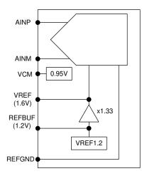
Figure 8-17. Different voltage reference options for ADC356x
