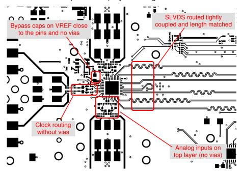
Figure 9-10. Layout example: top layer of ADC356x/368x EVM
