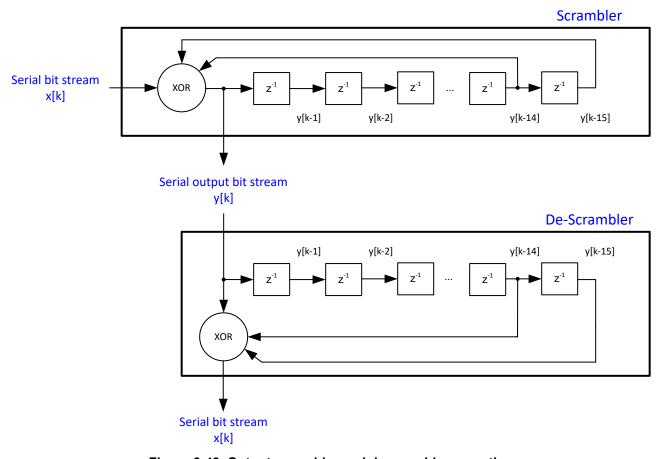
Figure 8-48. Output scrambler and descrambler operation
