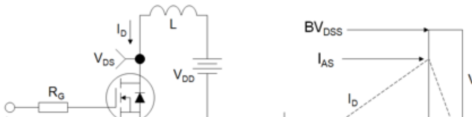
Figure C: Unclamped Inductive Switching Test Circuit and Waveform
