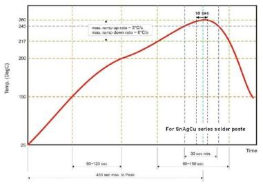
Fig 2. Infrared soldering profile
