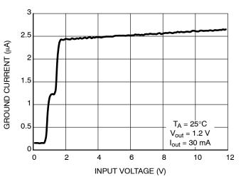
Figure 8. Ground Pin Current vs. Input Voltage
