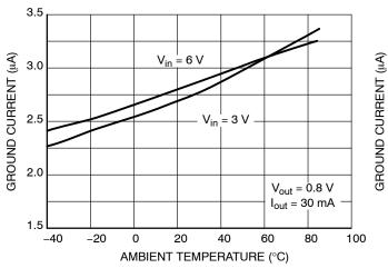
Figure 5. Ground Pin Current vs. Temperature
