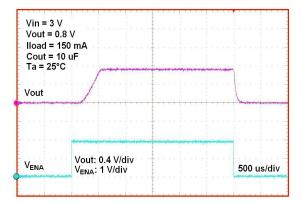
Figure 17. Enable Operation
