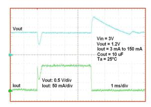
Figure 16. Load Transient Response
