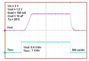
Figure 18. Enable Operation
