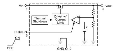
Figure 1. Representative Block Diagram
