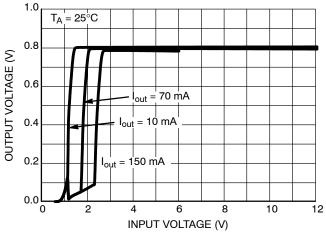
Figure 9. Output Voltage vs. Input Voltage
