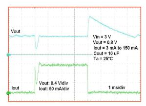
Figure 15. Load Transient Response
