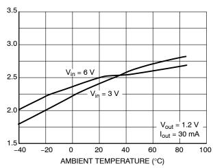
Figure 6. Ground Pin Current vs. Temperature
