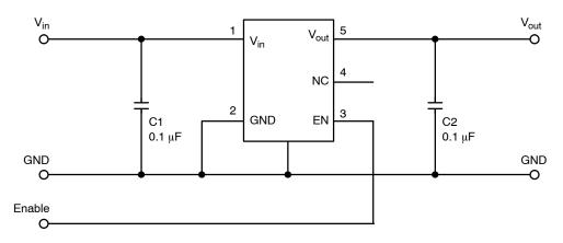
Figure 2. Typical Application Schematic for TSOP-5 Package
