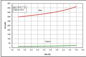
FIGURE 36-37: IPD, ADC Non-Converting, PIC16LF1615/9 Only.
