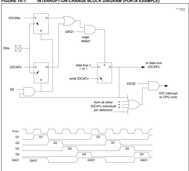
**FIGURE 14-1:** INTERRUPT-ON-CHANGE BLOCK DIAGRAM (PORTA EXAMPLE)
