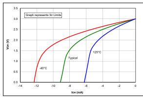
**FIGURE 36-45:** VOH vs. IOH Over Temperature, VDD = 3.0V.
