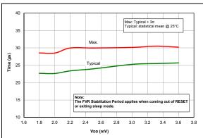
FIGURE 36-68: FVR Stabilization Period, PIC16LF1615/9 Only.
