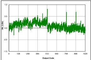
FIGURE 36-72: ADC 10-bit Mode, Single-Ended INL, VDD = 3.0V, TAD = 4  $\mu$ S, 25°C
