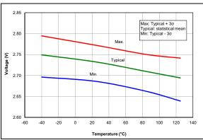
FIGURE 36-57: Brown-Out Reset Voltage, High Trip Point (BORV = 0).
