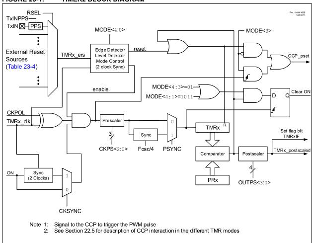
FIGURE 23-2: TIMER2 CLOCK SOURCE BLOCK DIAGRAM
