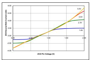
FIGURE 36-107: ZCD Pin Current over ZCD Pin Voltage, Typical Measured Values from -40°C to 125°C.
