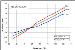
FIGURE 36-83: Temp. Indicator Slope
