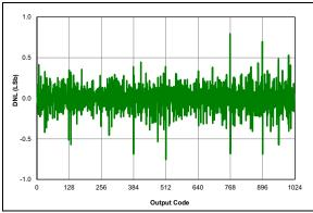
**FIGURE 36-69:** ADC 10-bit Mode, Single-Ended DNL, VDD = 3.0V,  $TAD = 1 \mu S$ ,  $25^{\circ}C$ .
