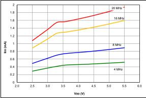
FIGURE 36-23: IDD Typical, HS Oscillator, 25°C, PIC16F1615/9 Only.
