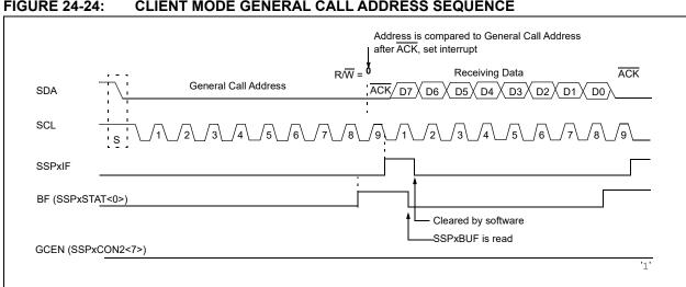
**FIGURE 24-24: CLIENT MODE GENERAL CALL ADDRESS SEQUENCE**
