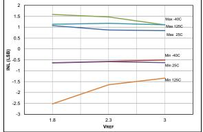
**FIGURE 36-76:** ADC 10-bit Mode, Single-Ended INL, VDD = 3.0V, TAD = 1  $\mu$ S.
