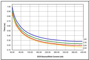
FIGURE 36-108: ZCD Pin Response Timer over Current, Typical Measured Values from -40°C to 125°C.
