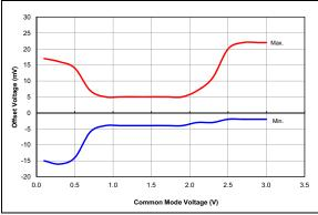
FIGURE 36-88: Comparator Offset, NP Mode (CxSP = 1), VDD = 3.0V, Typical Measured Values From -40°C to 125°C.
