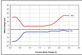
**FIGURE 36-87:** Comparator Offset, NP Mode (CxSP = 1), VDD = 3.0V, Typical Measured Values at 25°C.
