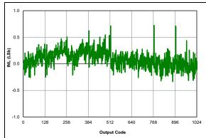
FIGURE 36-71: ADC 10-bit Mode, Single-Ended INL, VDD = 3.0V, TAD = 1  $\mu$ S, 25°C.
