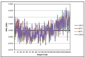
FIGURE 36-98: Typical DAC INL Error, VDD = 5.0V, VREF = External 5V, PIC16F1615/9 Only.
