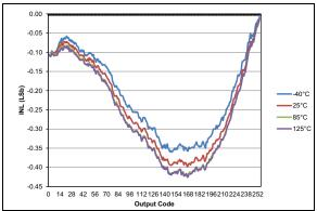
FIGURE 36-97: Typical DAC INL Error, VDD = 3.0V, VREF = External 3V.
