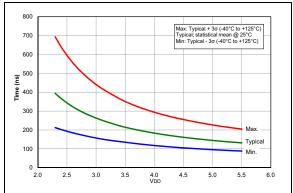
FIGURE 36-95: Comparator Output Filter
