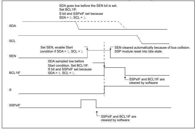
FIGURE 24-34: BUS COLLISION DURING START CONDITION (SCL = 0)
