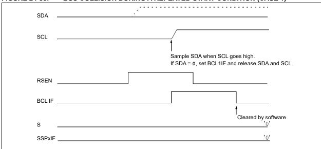
FIGURE 24-37: BUS COLLISION DURING REPEATED START CONDITION (CASE 2)
