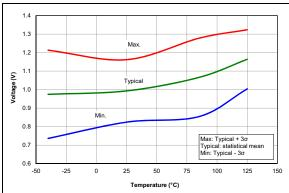
FIGURE 36-65: POR Rearm Voltage, NP Mode, PIC16LF1615/9 Only.
