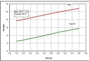
FIGURE 36-9: IDD Typical, EC Oscillator HP Mode, PIC16LF1615/9 Only.
