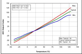
FIGURE 36-82: Temp. Indicator Slope
