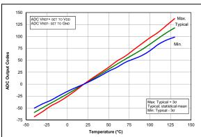
FIGURE 36-80: Temp. Indicator Slope
