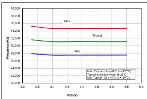
FIGURE 36-50: LFINTOSC Frequency, PIC16F1615/9 Only.
