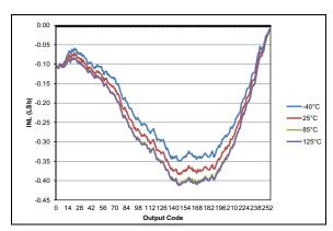
FIGURE 36-99: Typical DAC INL Error, VDD = 5.0V, VREF = External 5V, PIC16F1615/9 Only.
