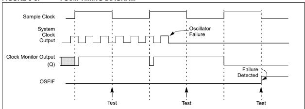
The system clock is normally at a much higher frequency than the sample clock. The relative frequencies in this example have been chosen for clarity.
