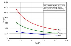
FIGURE 36-94: Comparator Output Filter
