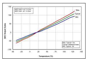
FIGURE 36-84: Temp. Indicator Slope
