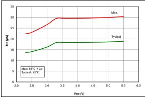
FIGURE 36-2: IDD, EC Oscillator LP Mode, Fosc = 32 kHz, PIC16F1615/9 Only.
