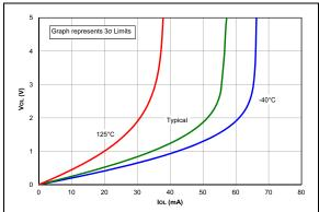
FIGURE 36-42: Vol. vs. Iol. Over
