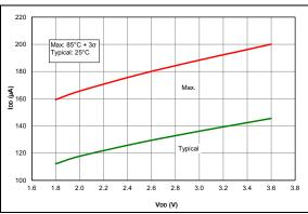
FIGURE 36-3: IDD, EC Oscillator LP Mode, Fosc = 500 kHz, PIC16LF1615/9 Only.
