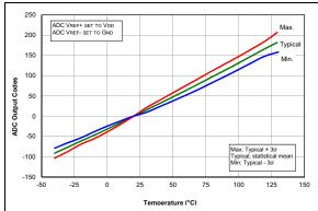
FIGURE 36-85: Temp. Indicator Slope
