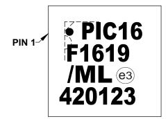
20-Lead QFN/UQFN (4x4x0.5 mm)
