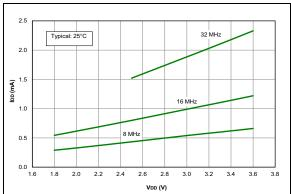
FIGURE 36-17: IDD Typical, HFINTOSC Mode, PIC16LF1615/9 Only.
