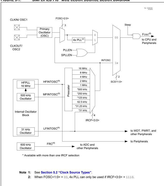
FIGURE 5-1: SIMPLIFIED PIC® MCU CLOCK SOURCE BLOCK DIAGRAM
