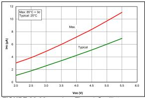
FIGURE 36-36: IPD, Timer1 Oscillator, Fosc = 32 kHz, PIC16F1615/9 Only.
