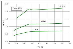
FIGURE 36-19: IDD Typical, HFINTOSC Mode, PIC16F1615/9 Only.
