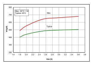
**FIGURE 36-39:** IPD, Comparator, NP Mode (CxSP = 1), PIC16LF1615/9 Only.
