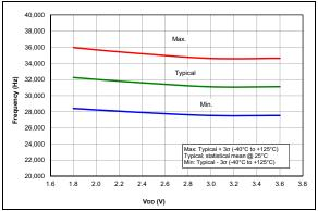
FIGURE 36-49: LFINTOSC Frequency, PIC16LF1615/9 Only.
