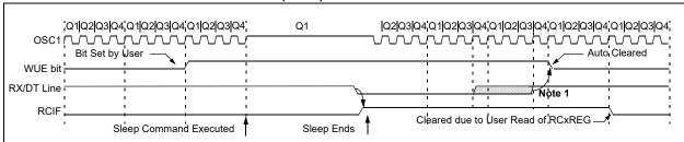
Note 1: If the wake-up event requires long oscillator warm-up time, the automatic clearing of the WUE bit can occur while the stposc signal is still active. This sequence must not depend on the presence of Q clocks.
