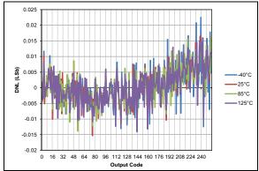
FIGURE 36-96: Typical DAC DNL Error, VDD = 3.0V, VREF = External 3V.
