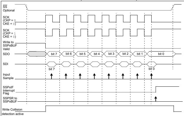
FIGURE 24-10: SPI MODE WAVEFORM (CLIENT MODE WITH CKE = 1)
