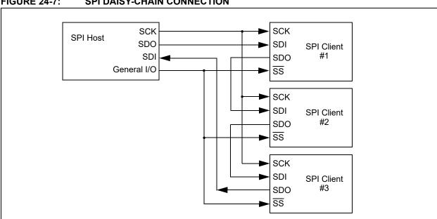
**FIGURE 24-7: SPI DAISY-CHAIN CONNECTION**
