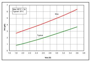
FIGURE 36-35: IPD, Timer1 Oscillator, Fosc = 32 kHz, PIC16LF1615/9 Only.
