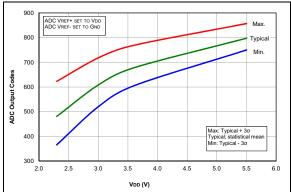
FIGURE 36-78: Temp. Indicator Initial Offset, Low Range, Temp. = 20°C, PIC16F1615/9 Only.
