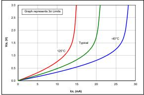
FIGURE 36-46: Vol. vs. Iol Over Temperature, VDD = 3.0V.
