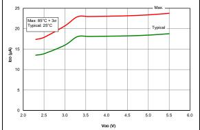
FIGURE 36-106: ZCD Response Time over Voltage Typical Measured Values.
