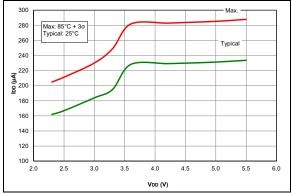
FIGURE 36-4: IDD, EC Oscillator LP Mode, Fosc = 500 kHz, PIC16F1615/9 Only.
