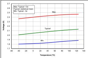
FIGURE 36-59: LPBOR Reset Voltage.
