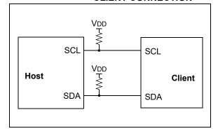
The Acknowledge bit  $(\overline{ACK})$  is an active-low signal, which holds the SDA line low to indicate to the transmitter that the client device has received the transmitted data and is ready to receive more.
