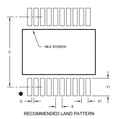
Units MILLIMETERS Dimension Limits MIN NOM MAX Contact Pitch 0.65 BSC Ε С Contact Pad Spacing 7.20 Contact Pad Width (X20) X1 0.45 Contact Pad Length (X20) Y1 1.75 Distance Between Pads G 0.20
