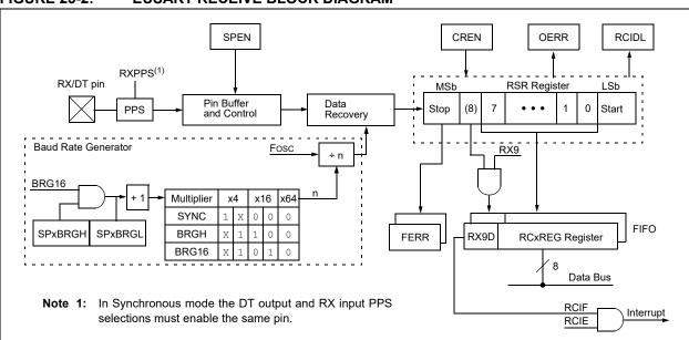
FIGURE 25-2: EUSART RECEIVE BLOCK DIAGRAM
