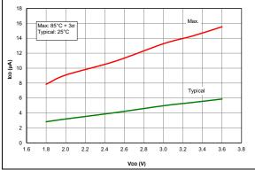
FIGURE 36-1: IDD, EC Oscillator LP Mode, Fosc = 32 kHz, PIC16LF1615/9 Only.
