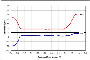
**FIGURE 36-90:** Comparator Offset, NP Mode (CxSP = 1), VDD = 5.0V, Typical Measured Values at 25°C, PIC16F1615/9 Only.
