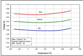
FIGURE 36-63: POR Release Voltage.
