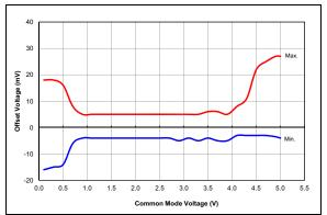
FIGURE 36-91: Comparator Offset, NP Mode (CxSP = 1), VDD = 5.5V, Typical Measured Values From -40°C to 125°C, PIC16F1615/9 Only.
