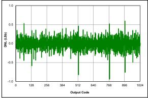
**FIGURE 36-70:** ADC 10-bit Mode, Single-Ended DNL, VDD = 3.0V,  $TAD = 4 \mu S$ ,  $25^{\circ}C$ .
