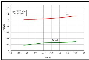
FIGURE 36-38: IPD, ADC Non-Converting, PIC16F1615/9 Only.
