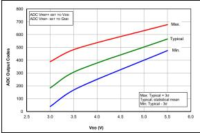
FIGURE 36-77: Temp. Indicator Initial Offset, High Range, Temp. = 20°C, PIC16F1615/9 Only.
