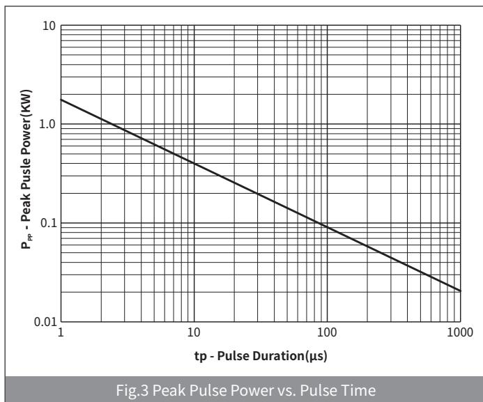
Fig.3 Peak Pulse Power vs. Pulse Time
