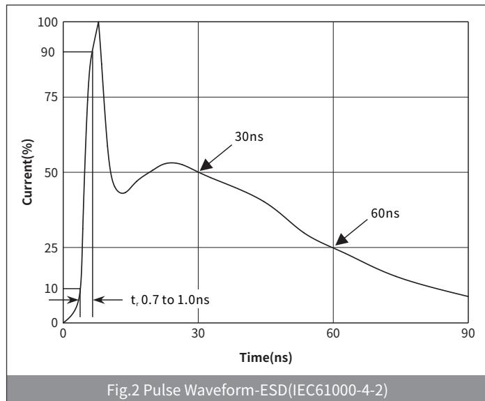
Fig.2 Pulse Waveform-ESD(IEC61000-4-2)
