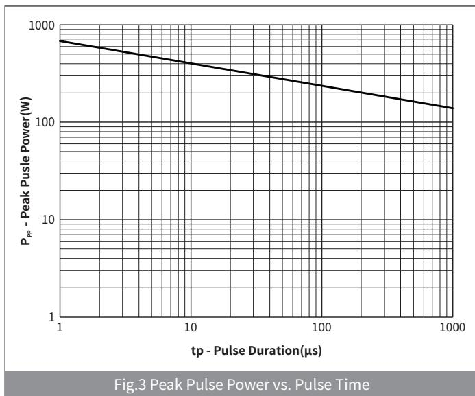
Fig.3 Peak Pulse Power vs. Pulse Time
