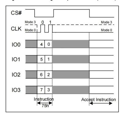
Figure 7.19b Erase / Program Suspend Instruction (QPI Mode)
