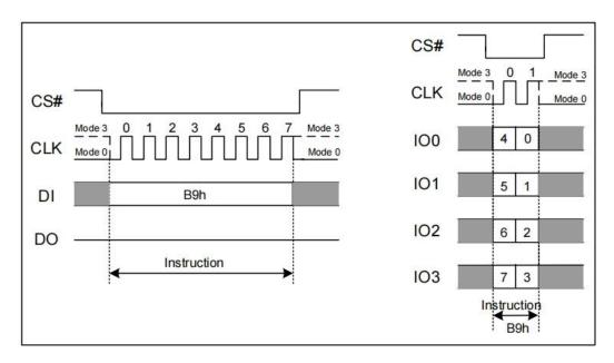
Figure 7.37 Deep Power-down Instruction(SPI and QPI Mode)
