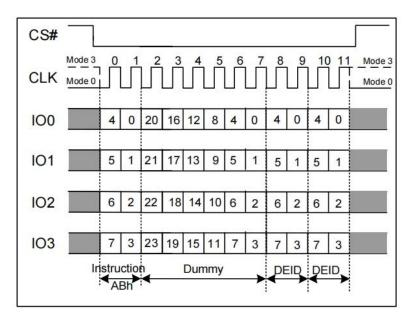
Figure 7.38c Release Power-down / Device ID(QPI Mode)
