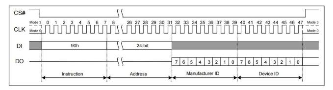
Figure 7.39 Read Manufacturer/Device ID (SPI Mode)
