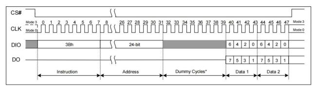
Figure 7.26 Fast Read Dual Output Instruction Sequence Diagram (SPI Mode only)
