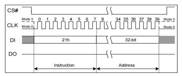
Figure 7.15 Sector Erase with 4-Byte Address Instruction (SPI Mode Only)
