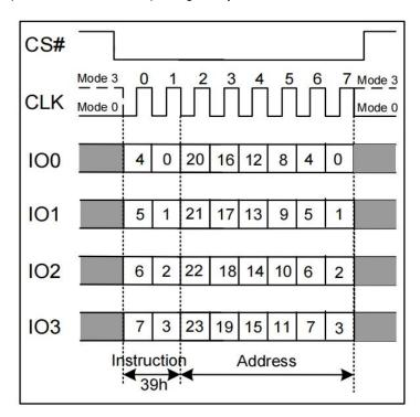
Figure 7.49b Individual Block/Sector Unlock Instruction(QPI Mode)
