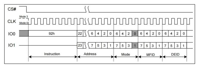
Figure 7.25 Read Manufacturer/Device ID Dual I/O Instruction
