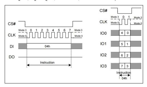
Figure 7.4 Write Disable Instruction (SPI or QPI Mode)
