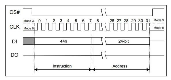
Figure 7.44 Erase Security Registers Instruction (SPI Mode only)
