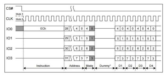
Figure 7.34a Fast Read Quad I/O with 4-Byte Address Instruction (M7-0 = FFh, SPI Mode)
