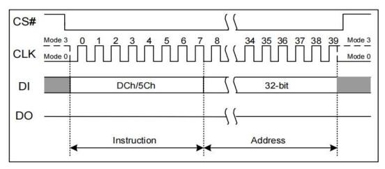
Figure 7.17 Block Erase with 4-Byte Address Instruction (SPI Mode Only)
