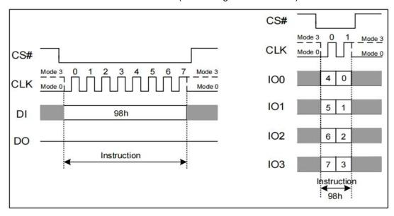
Figure 7.24 Global Block Lock Instruction(SPI or QPI Mode)
