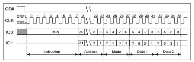
Figure 7.31a Fast Read Dual I/O with 4-Byte Address (Initial command or previous M5-4≠10, SPI Mode only)
