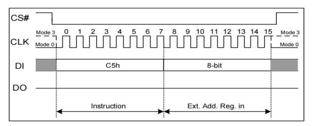
Figure 7.7a Write Extended Address Register Instruction (SPI Mode)
