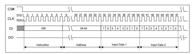
Figure 7.45 Program Security Registers Instruction (SPI Mode only)
