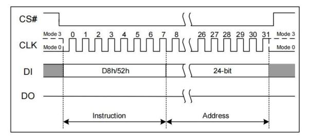
Figure 7.16a Block Erase Instruction(SPI Mode)
