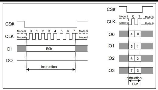
Figure 7.38 a Release Power-down Instruction(SPI and QPI Mode)
