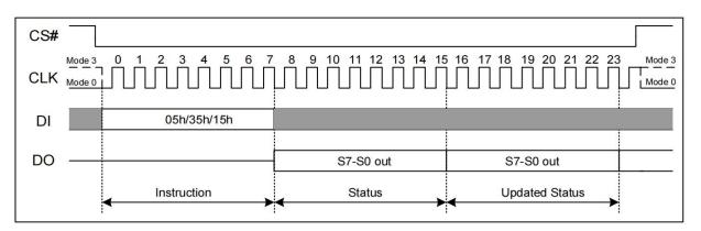
Figure 7.1a Read Status Register Instruction (SPI Mode)
