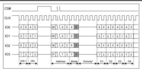
Figure 7.34b Fast Read Quad I/O with 4-Byte Address (Previous instruction set M5-4 = 10, SPI Mode)
