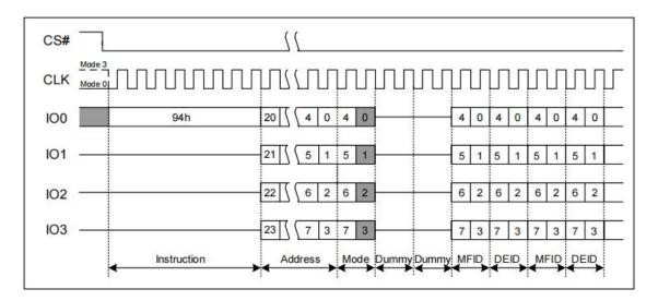
Figure 7.26 Read Manufacturer/Device ID Quad I/O Instruction
