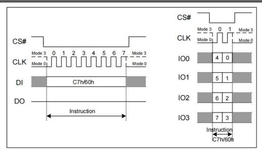
Figure 7.18 Chip Erase Instruction(SPI or QPI Mode)
