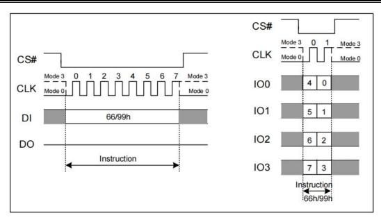
Figure 7.36 Software Reset Instruction(SPI and QPI Mode)
