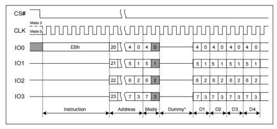
Figure 7.32a Fast Read Quad I/O Instruction (Initial command or previous M5-4#10, SPI Mode)
