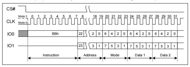
Figure 7.30a Fast Read Dual I/O Instruction (M7-0=FFh, SPI Mode only)
