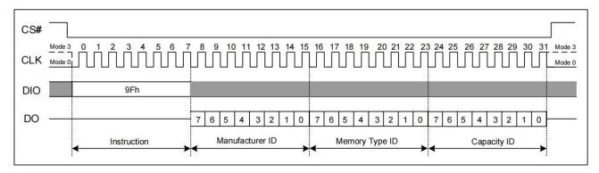
Figure 7.41 Read JEDEC ID(SPI Mode)
