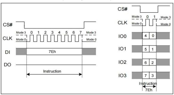
Figure 7.51 Global Block Lock Instruction(SPI or QPI Mode)
