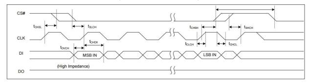
Figure 8.5 Input Timing
