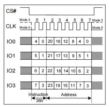
Figure 7.48 Individual Block/Sector Lock Instruction(QPI Mode)
