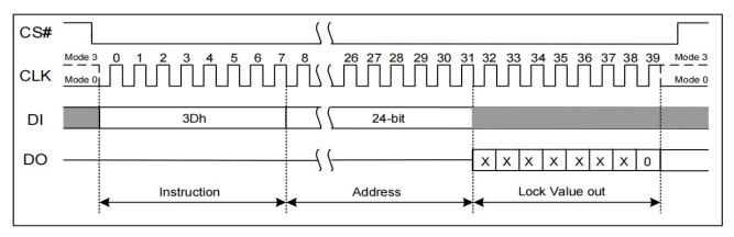
Figure 7.50a Read Block Lock Instruction(SPI Mode)
