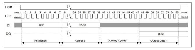
Figure 7.25 Fast Read with 4-Byte Address Instruction (SPI Mode only)
