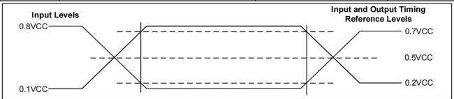
Figure 8.3 AC Measurement I/O Waveform
