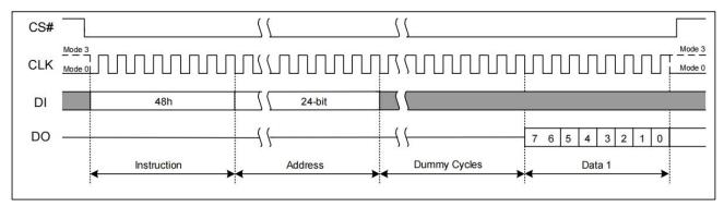
Figure 7.46 Read Security Registers Instruction (SPI Mode only)
