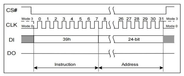
Figure 7.49 Individual Block/Sector Unlock Instruction(SPI Mode)
