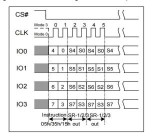
Figure 7.1b Read Status Register Instruction (QPI Mode)
