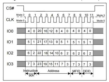
Figure 7.40 Read Manufacturer/Device ID (QPI Mode)
