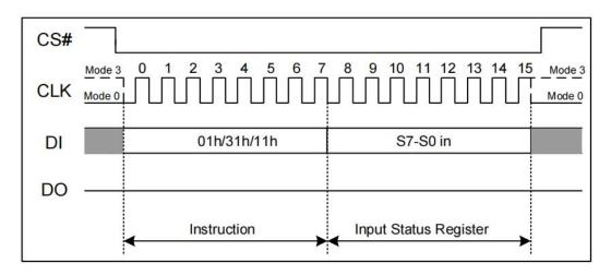
Figure 7.5a Write Status Register Instruction(SPI Mode)
