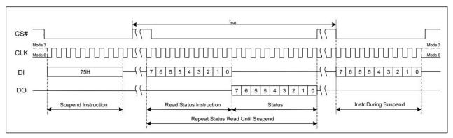
Figure 7.19a Erase / Program Suspend Instruction (SPI Mode)
