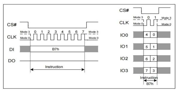
Figure 7.8 Enter 4-Byte Address mode Instruction (SPI or QPI Mode)
