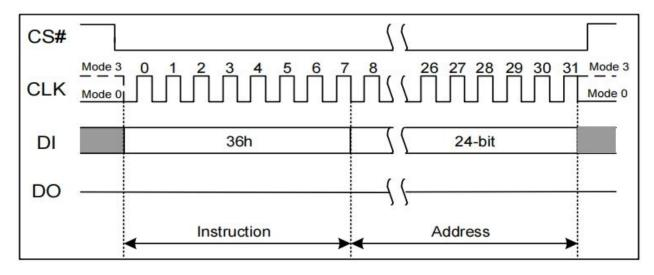
Figure 7.47 Individual Block/Sector Lock Instruction(SPI Mode)
