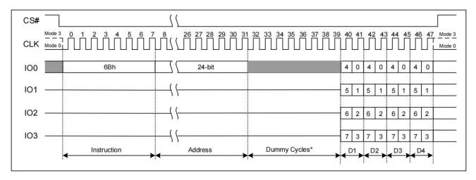
Figure 7.28 Fast Read Quad Output Instruction (SPI Mode only)
