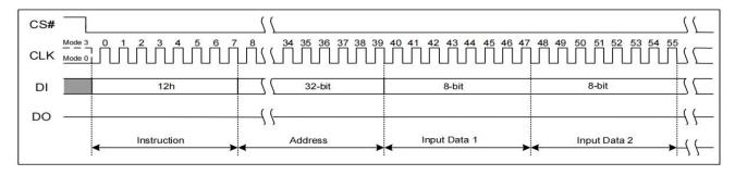
Figure 7.11 Page Program with 4-Byte Address Instruction (SPI Mode Only)
