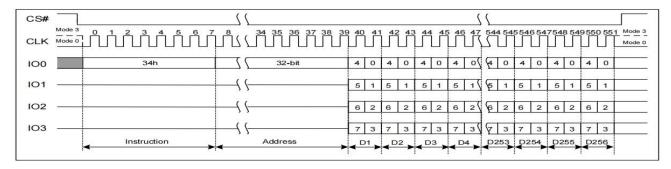
Figure 7.13 Quad Input Page Program with 4-Byte Address Instruction (SPI Mode only)
