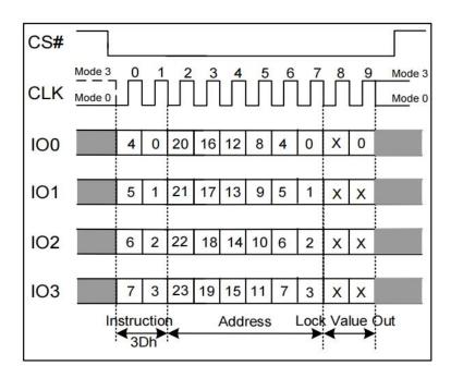
Figure 7.50b Read Block Lock Instruction(QPI Mode)
