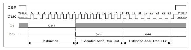
Figure 7.6a Read Extended Address Register Instruction (SPI Mode)
