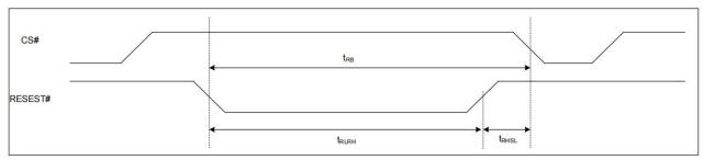
Figure 8.8 Hardware Reset Timing
