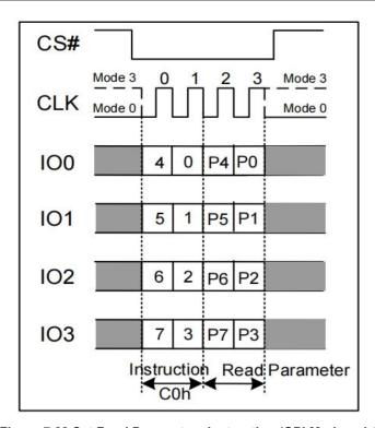
Figure 7.28 Set Read Parameters Instruction (QPI Mode only)
