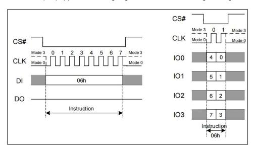
Figure 7.2 Write Enable Instruction (SPI or QPI Mode)
