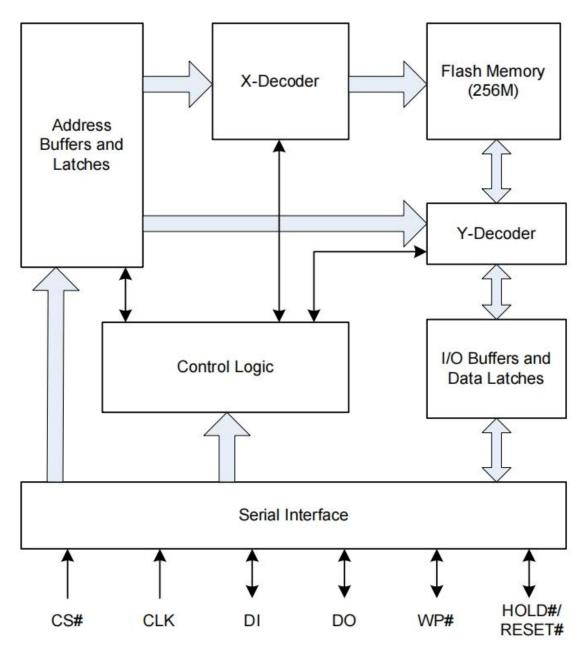
Figure 2.1 Block Diagram
