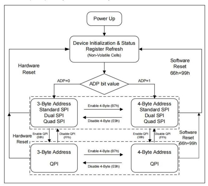
Figure 6.2 HG25Q256 Serial Flash Memory Operation Diagram
