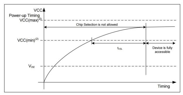
Figure 8.1 Power-up Timing
