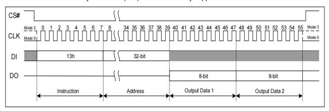
Figure 7.22 Read Data with 4-Byte Address Instruction (SPI Mode only)
