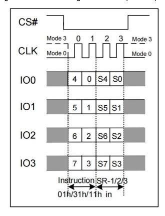
Figure 7.5b Write Status Register Instruction (QPI Mode)
