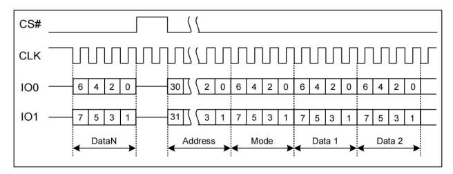
Figure 7.31b Fast Read Dual I/O with 4-Byte Address (Previous M5-4=10, SPI Mode only)
