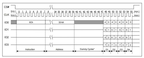
Figure 7.29 Fast Read Quad Output with 4-Byte Address Instruction(SPI Mode only)
