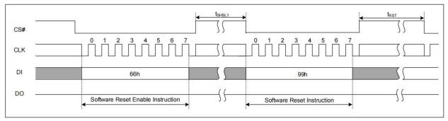
Figure 8.7 Software Reset Input Timing
