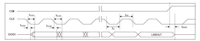
Figure 8.4 Serial Output Timing
