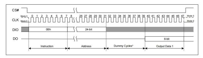
Figure 7.23 Fast Read Instruction (SPI Mode)
