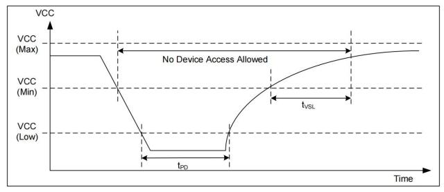
Figure 8.2 Power-Down and Voltage Drop
