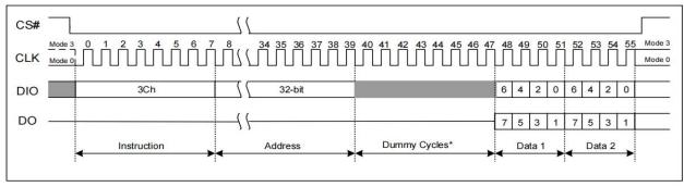
Figure 7.27 Fast Read Dual Output with 4-Byte Address Instruction (SPI Mode only)
