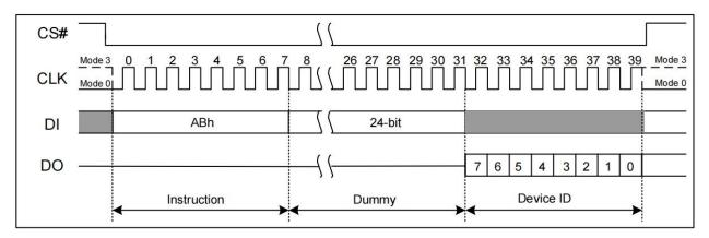
Figure 7.38b Release Power-down / Device ID(SPI Mode)
