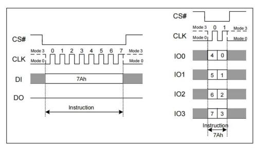
Figure 7.20 Erase/Program Resume Instruction(SPI or QPI Mode)
