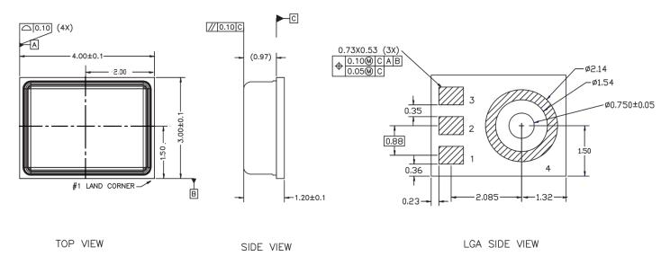
Figure 11. 4-Terminal Chip Array Small Outline No Lead Cavity 4 mm  $\times$  3 mm  $\times$  1.2 mm Dimensions shown in millimeters
