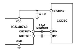
Figure 8. ICS-40740 Connected to a Codec
