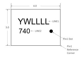
Figure 12. Package Marking Specification (Top View)
