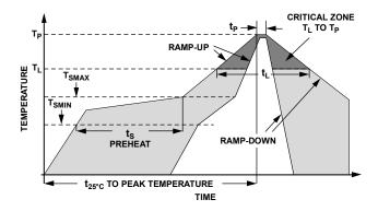
Figure 1. Recommended Soldering Profile Limits
