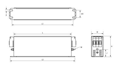
**General Information** Series FLLD3-MH Style **Chassis Mount** Description EMI Filter, Chassis Mount, Motor Drives Three Phase, High Performance, High Voltage Features Phase Three-phase RoHS Yes Qualifications IEC/EN 60939, UL 1283 **Terminal Type** Threaded Studs M6
