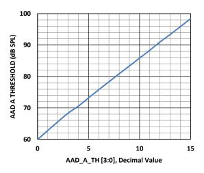
Figure 11 AAD Analog Threshold vs Register Value
