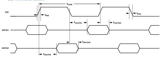
Figure 1. Pulse Density Modulated Output Timing
