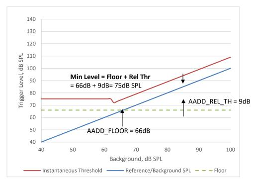
Figure 25. Relative Threshold with floor indicated
