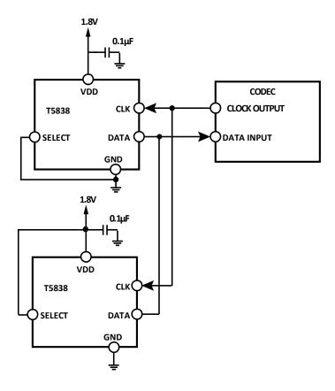
Figure 30. Stereo PDM Microphone Connection to Codec
