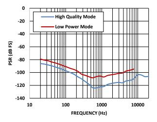
Figure 8. PSR vs Frequency
