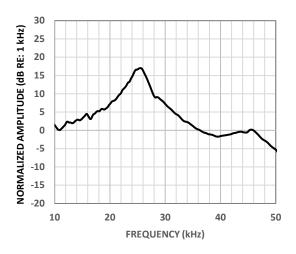
Figure 9. Typical Ultrasonic Frequency Response, Ultrasonic Mode
