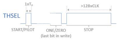
Figure 20. Write termination with Stop High
