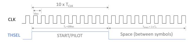
Figure 21. Timing diagram for example above showing relationship between THSEL pilot and CLK
