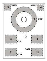
Figure 3. Pin Configuration (Top View, Terminal Side Down)
