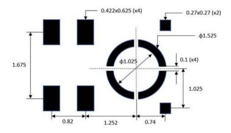
Figure 33. Suggested Solder Paste Stencil Pattern Layout
