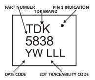
Figure 35. Package Marking Specification (Top View)
