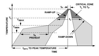
**Figure 2. Recommended Soldering Profile Limits**
