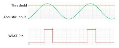
Figure 23. AAD A Threshold level and WAKE pin activation.
