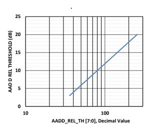
Figure 13. AAD Digital 1,2 Relative Threshold vs Register Value
