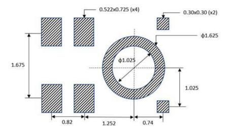
Figure 32. Recommended PCB Land Pattern Layout
