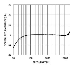
Figure 4. Typical Audio Frequency Response, High Quality Mode
