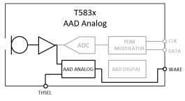
Figure 16. Block Diagram for AAD Analog Operation
