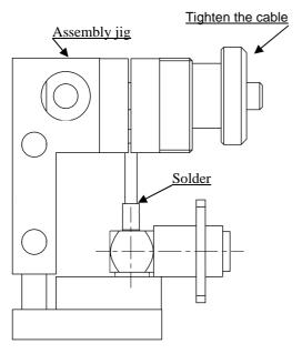
After cooling, remove the assembly from the jig. Solder the inner conductor. Place the cap into the body. Press on the cap flush or slightly below the surface of the body assembly.
