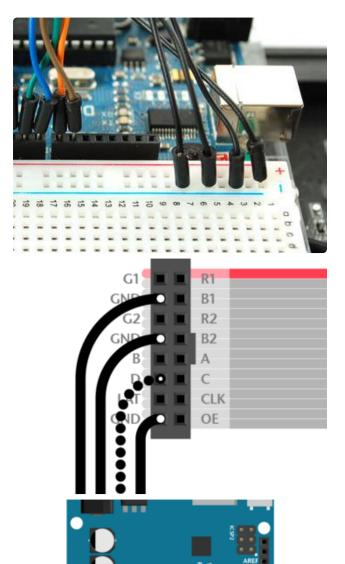
32x32 and 64x32 matrices require three ground connections. 32x16 matrices have four.
