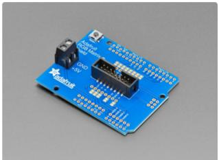
The included headers should be installed from the underside and soldered from the top.
