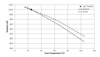
**Figure 8: Derating Curve**
