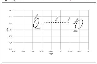
Figure 4: Color Shift vs. Forward Current 3000K - 1800K
