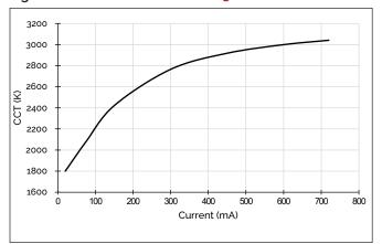
Figure 3: Color Shift vs. Forward Current 2700K - 1800K
