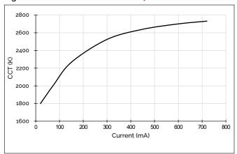
Figure 2: CCT vs. Forward Current 3000K-1800K
